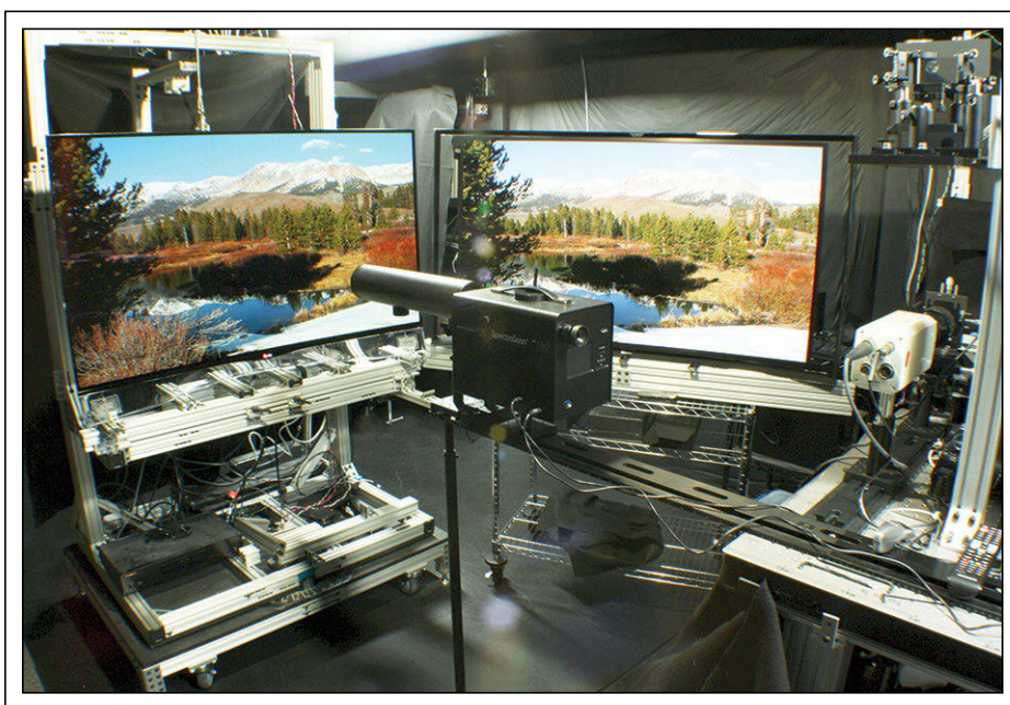
Fig. 1: The LG 55EA9800 and the Samsung KN55S9CAFXZA 55-in. curved OLED TVs were tested for this article. The LG is at the left and is mounted for measurement. A photograph is shown on the displays for visual interest, but patterns were used for measurements.
