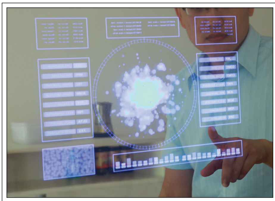
Fig. 5: The display shown uses a transparent and water-clear EPD based on DLP projection with a UHP lamp source.
