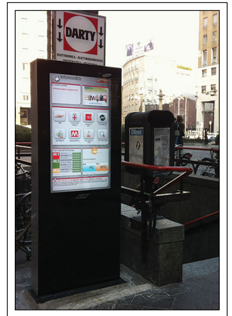
Fig. 1: This interactive kiosk-type LCD is connected to Milan’s transport system and offers a touch interface for users to find information on train schedules, weather, and events.
