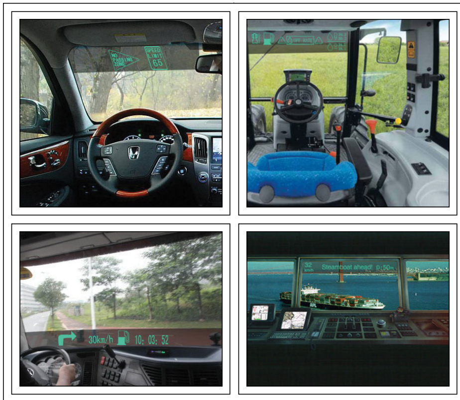
Fig. 11: The current EPD HUD product as shown in Fig. 10 can be readily implemented onto various vehicle windshields, including (clockwise) cars, tractors, trucks, and ships.
