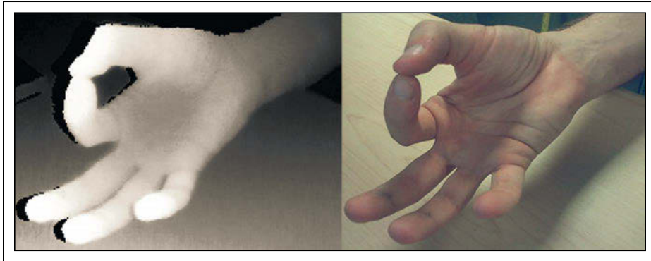
Fig. 1: Shown at left is the output from a 3D imaging device, with depth mapping that shows nearer points as brighter. At right is the corresponding color image.
