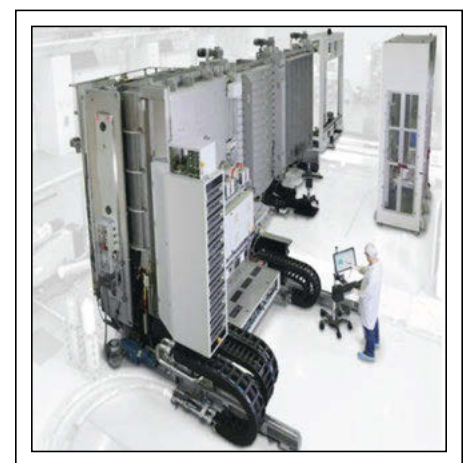
Fig. 3: The AKT-PiVot 55K DT PVD system is designed for manufacturing large-area ultra-high-definition LCD and OLED panels.
