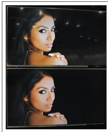
Fig. 3: BenQ Material's True Black Functional Film (bottom) reduces ambient reflections and internal light leakage, as compared to the top image without the film. Photo: Ken Werner
