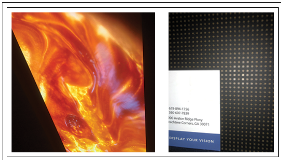
Fig. 1: The author attended a showing of Avengers: Infinity War on one of the new Samsung 4K LED “Onyx” screens at the Pacific Theatres Winnetka in Chatsworth, California. The imagery was impressive (left). At right, a business card is compared to the pixel arrays in the theater screen. All photos by Gary Feather
