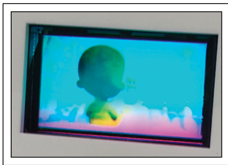
Fig. 2: Hong Kong University of Science and Technology’s 3-in. diagonal, 250-ppi active-matrix field-sequential color display featured an ultra-fast response time of \sim 10 \mu\text{s} . Photo: Steve Sechrist
