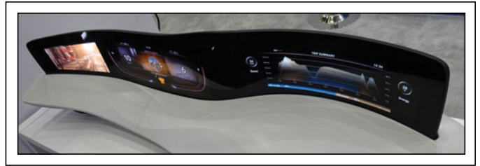
Fig. 4: Continental and AGC teamed up for a curved hot-formed glass display with two 12.3-in. OLEDs and one 7-in. OLED.
