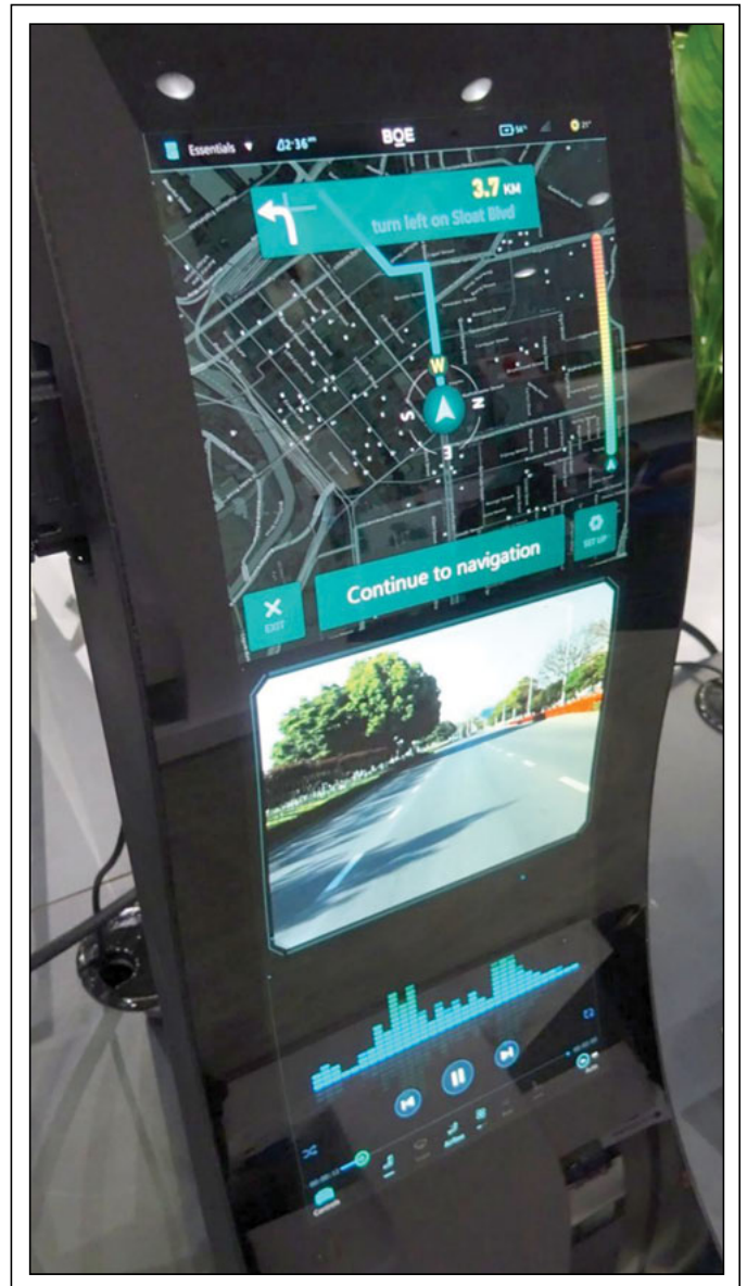
Fig. 11: This thin (0.5 mm) flexible 12.3-in. OLED from BOE features 600 \text{ cd/m}^2 , a wide color gamut, and a power consumption of 14 W.
