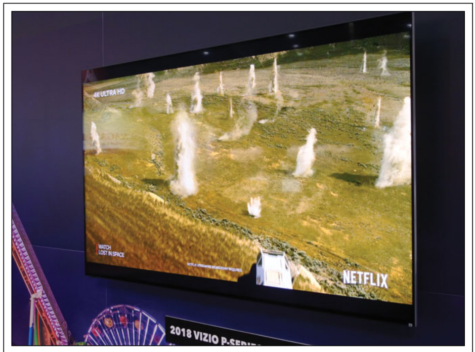
Fig. 3: The Vizio P Series Quantum TV with Nanosys's Hyperion QD film and 192 full-array local dimming zones delivered an impressive image. Photo: Ken Werner
