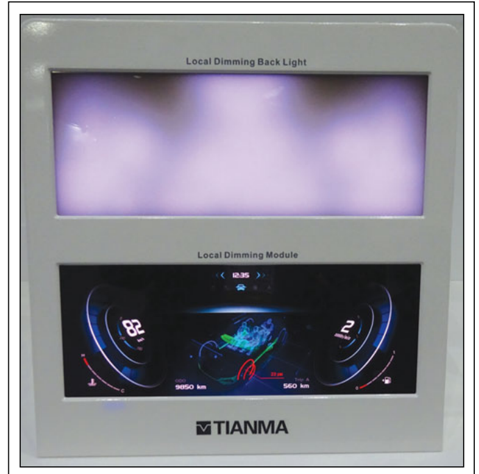
Fig. 8: This visualization of local direct dimming by Tianma with 240 segments (LEDs) resulted in a dynamic contrast ratio over 40 million to 1 and consumes power at reference images only about 1/3 of the electrical power of a standard panel.
