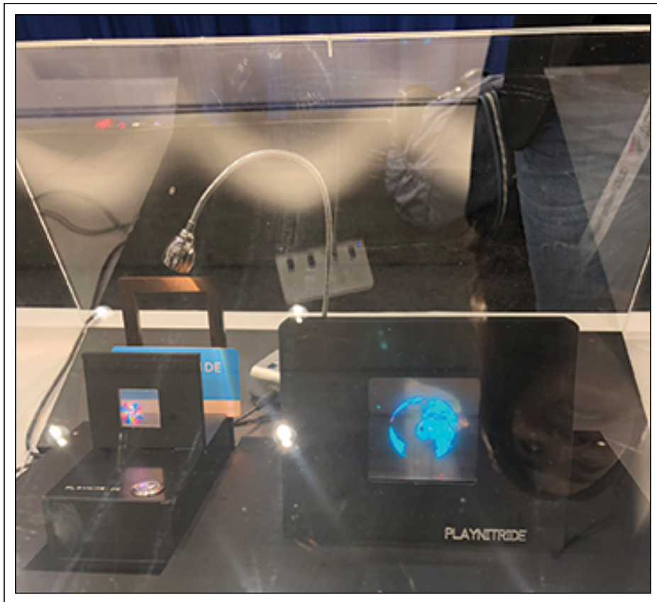
Fig. 5: PlayNitride's transparent microLED display was 3.12 inches diagonal, with a luminance of more than 800 cd/m 2 . Photo: Steve Sechrist
