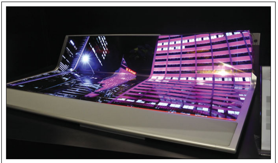
Fig. 1: LGD's 77-in. flexible OLED screen with 8 million pixels and 40 percent transmittance greeted attendees at the Display Week exhibition. Photo: Ken Werner
