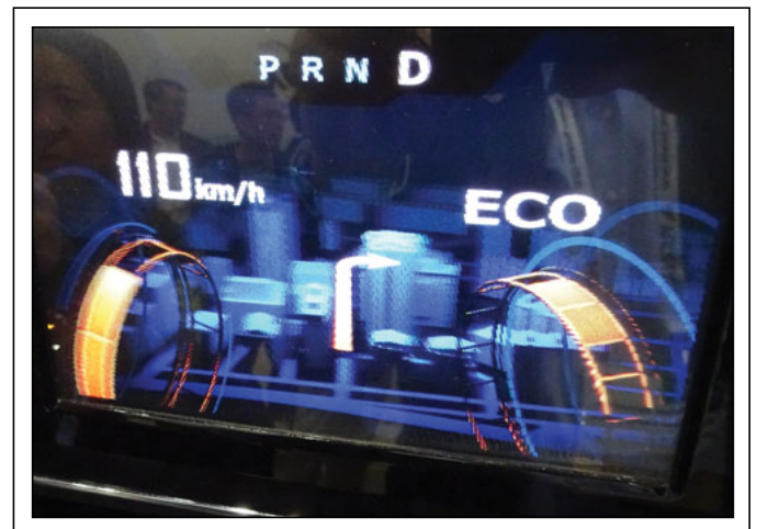
Fig. 9: This picture shows an automotive autostereoscopic 3D light-field based display with 18 views by Samsung. This 7-in. WXGA OLED enables a 3D depth of 80 mm in total.
