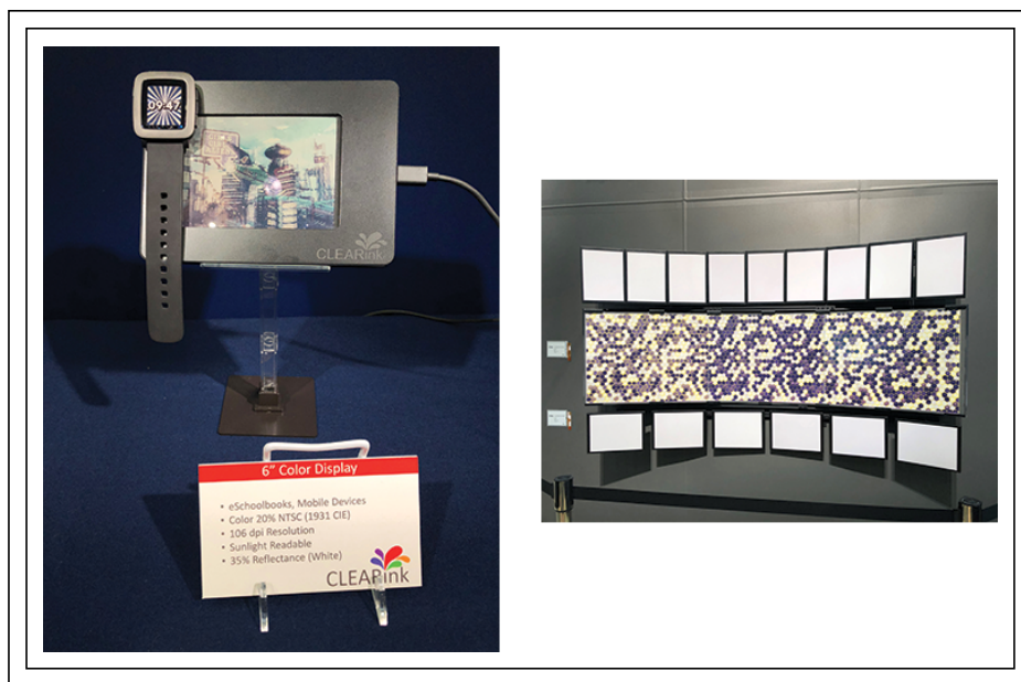
Fig. 2: CLEARink’s reflective color display (left) is designed to offer video-level refresh rates. At right, E Ink was demonstrating color panels at Display Week that could be tiled and updated to provide a large, changing display.
