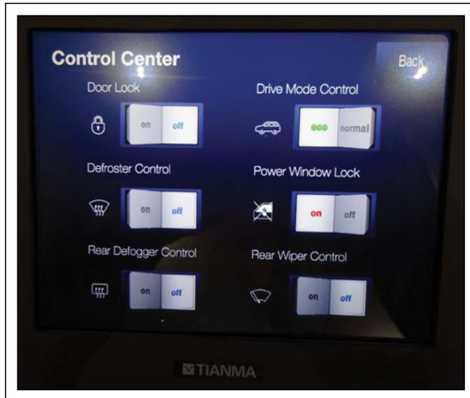
Fig. 12: This electrostatic tactile touch display by Tianma improves safety for automotive use compared to standard touch. Both texture (e.g., rough surface) and click (a feeling similar to a mechanical push button) sensations are possible.
