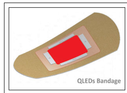
Fig. 3. A QLED-based bandage for photomedicine applications might look like the rendering above.
