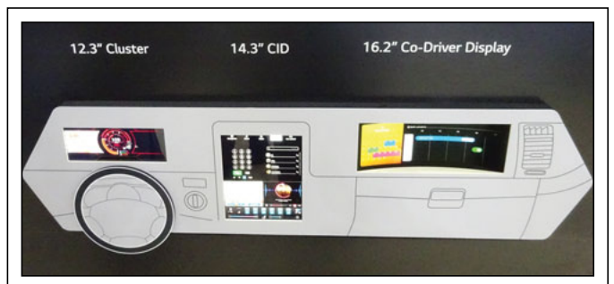
Fig. 5: This demo includes examples of LG’s automotive LTPS LCDs with high luminance ( 1,000 \text{ cd/m}^2 ) and about 200 ppi. The center display sports an in-cell touch while the co-driver display achieves a dynamic contrast ratio of 100,000:1 by local dimming.
