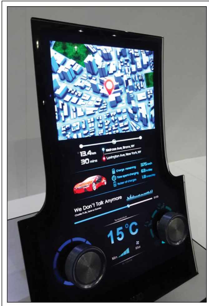
Fig. 10: This 13.2-in. center-stack freeform LCD from AUO has two symmetrical holes of 35-mm diameter that enable easy integration of mechanical rotary knobs. Other features are a curvature of 1,000 mm, a-Si gate driver integrated within the display area, 1,000 \text{ cd/m}^2 and a resolution of 1,600 \times 1,200 .
