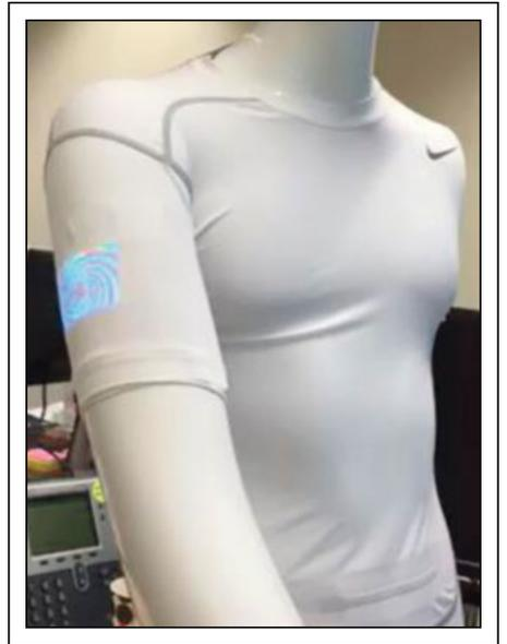
**Fig. 2:** This conformable  $64 \times 45$  RGB LED matrix is integrated into the sleeve of a t-shirt that is mounted on a mannequin. Source: IMEC, Ghent University, Holst/TNO, and Panasonic; 2016 SID Digest of Technical Papers.
