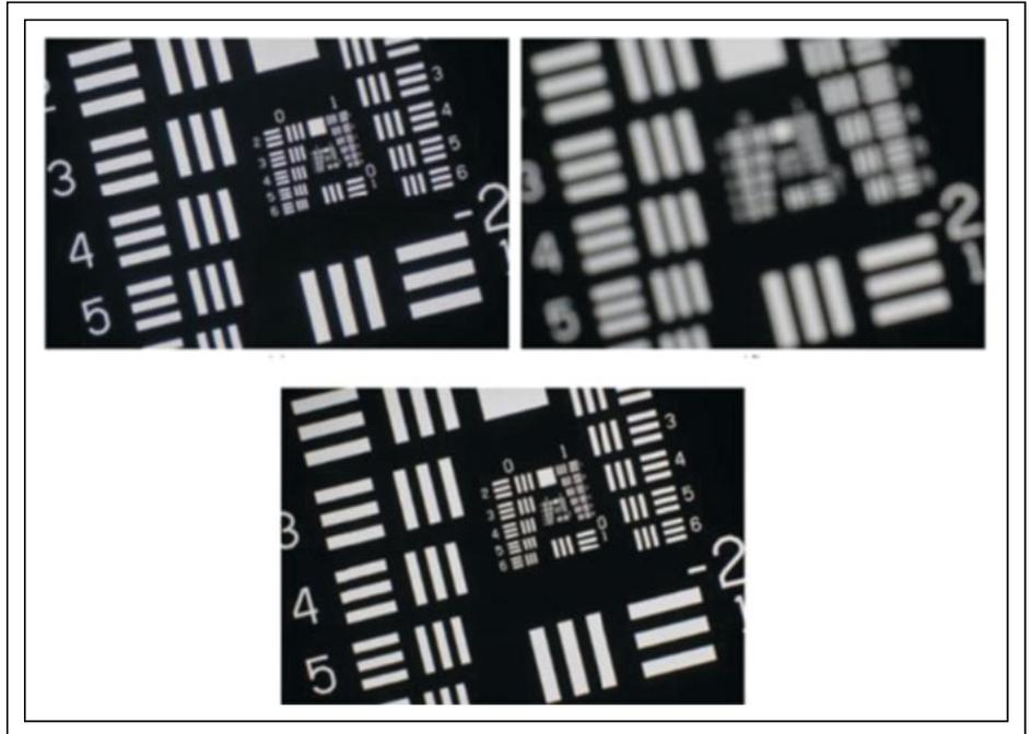
**Fig. 3:** Results from an adjustable liquid-crystal lens include a lens image taken with voltage applied to provide a 400-mm focal length to focus the image (top left), an LC lens image with 0 V applied (right), and a glass lens image with a 400-mm focal length for reference (bottom).<sup>5</sup>
