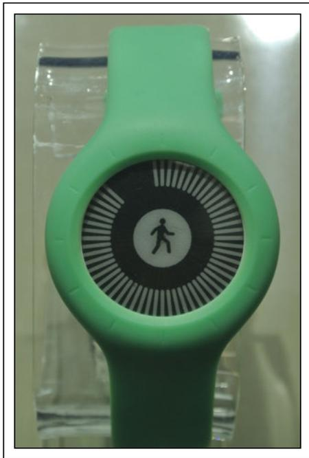
*Fig. 7: The Withings activity monitor device uses an electronic-ink screen. Photo courtesy Jyrki Kimmel.*
