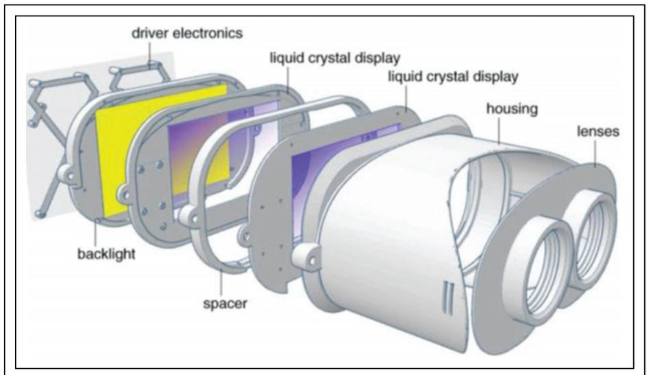
**Fig. 4:** A prototype light-field stereoscope comprising two stacked LCD panels.<sup>3</sup>
