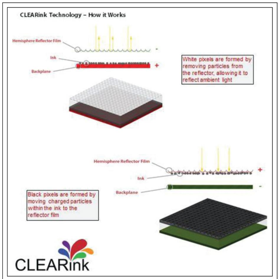
*Fig. 2: CLEARink's innovative electrophoretic architecture enables a much faster response time – even supporting video imagery.*
