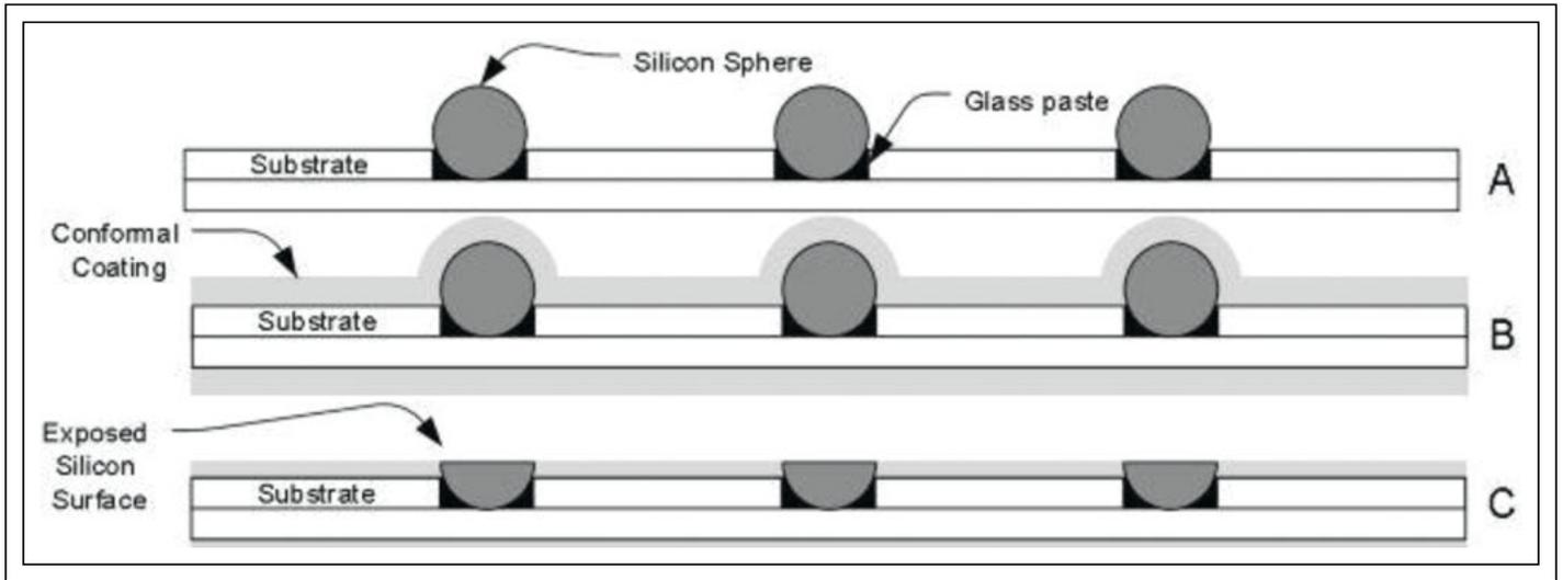
**Fig. 3:** Single-crystal-silicon spheres are embedded in a ceramic substrate that is then planarized at the surface in an approach that could be used to make large-area substrates with high mobility. Source: R. S. Tarighat et. al.
