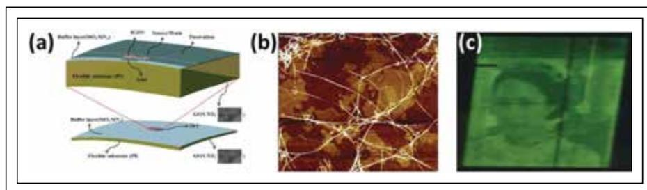
**Fig. 1:** A plastic AMOLED display with gate-driver-in-panel (GIP) is depicted in several views: (a) cross-sectional view, (b) CNT/GO TEM image at the back side of PI substrate, and (c) green AMOLED image on PI substrate with pixel size of 30  $\mu\text{m}$   $\times$  30  $\mu\text{m}$  and integrated gate driver using BA a-IGZO TFTs. An AMOLED display driven by a 30- $\mu\text{m}$ -pitch integrated gate driver is shown.<sup>1,2</sup>
