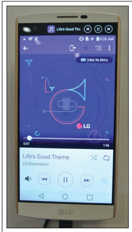
**Fig. 2:** LG Display's 6.0-in. dual-driver QHD+ mobile display had a 160-pixel extra screen strip at the top, leaving the bottom as the "normal" smartphone screen. Photo courtesy Jyrki Kimmel.
