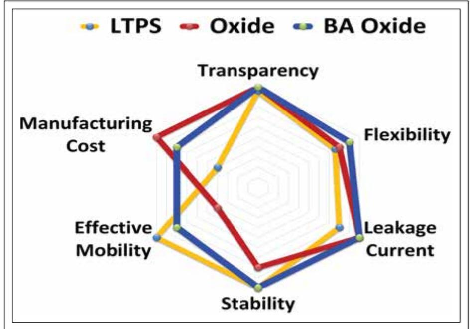
Fig. 3: The schematic illustrates a comparison among LTPS, oxide, and BA-oxide TFTs for flexible-display applications. The BA-TFT backplane has the advantages of manufacturing cost, flexibility, leakage current, and transparency compared to that of LTPS TFTs.
