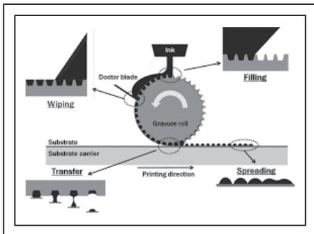
**Fig. 1:** In this conceptual view of gravure printing, ink is dispensed to fill wells in the gravure cylinder. Excess ink is wiped using a doctor blade. Ink is transferred to a passing substrate; the ink subsequently spreads and dries. Source: UC Berkeley; 2016 SID Digest of Technical Papers.
