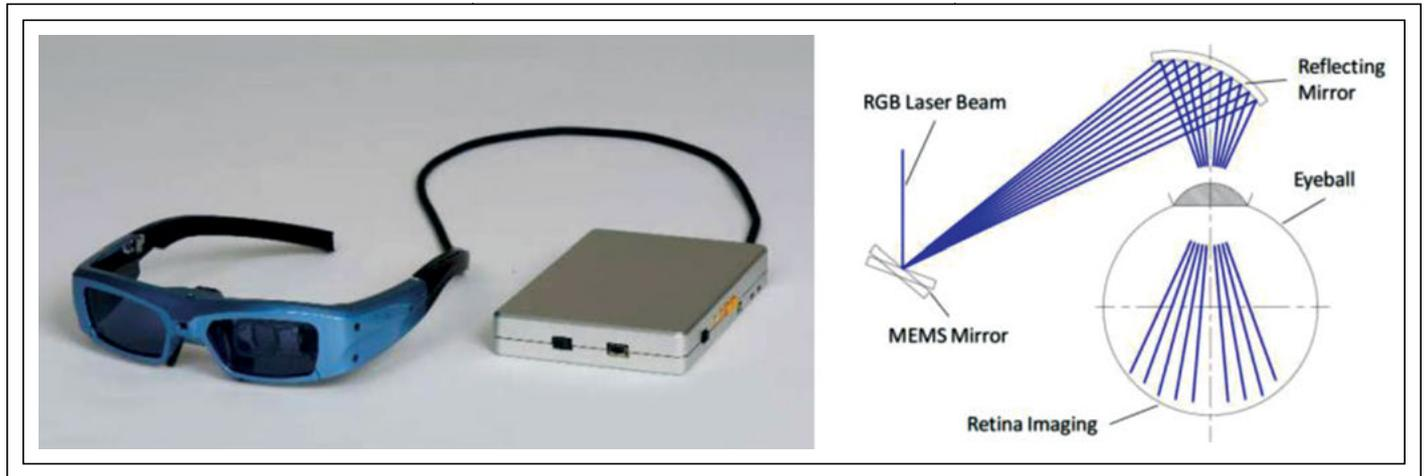
**Fig. 5:** This retinal imaging laser eyewear incorporates an asymmetric free-surface mirror.<sup>8</sup>
