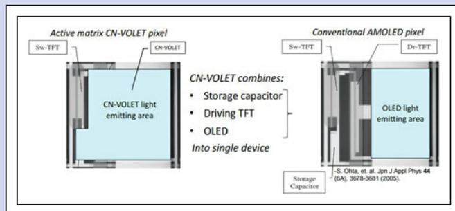
**Fig. 3:** nVerpix's carbon-nanotube-vertical OLED light-emitting transistor (left) can deliver a much larger aperture ratio than a conventional AMOLED (right).
