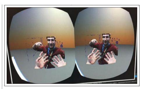
**Fig. 7:** The "merged reality "capability of a device is shown here with integrated Intel RealSense technology.<sup>10</sup> The 3D images of the user's hands as well as a person standing in front of the user are brought into the virtual world. This capability is also used to allow multiroom scale mobility with integrated six degrees-of-freedom positional tracking to help the user avoid colliding with physical objects.
