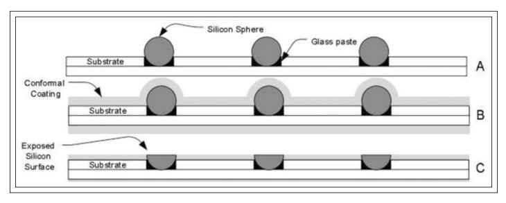
*Fig. 3:* Single-crystal-silicon spheres are embedded in a ceramic substrate that is then planarized at the surface in an approach that could be used to make large-area substrates with high mobility. Source: R. S. Tarighat et. al.
