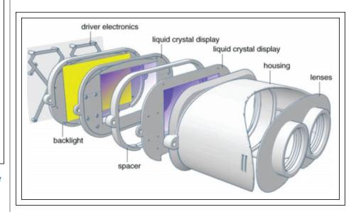
Fig. 4: A prototype light-field stereoscope comprising two stacked LCD panels.<sup>3</sup>
