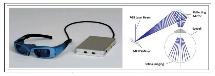
Fig. 5: This retinal imaging laser eyewear incorporates an asymmetric free-surface mirror.<sup>8</sup>
