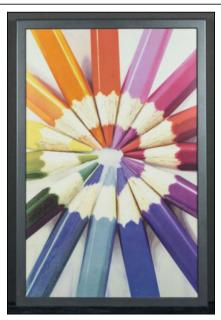
**Fig. 3:** *E* Ink's new color electrophoretic technology produces color without the use of filters.
