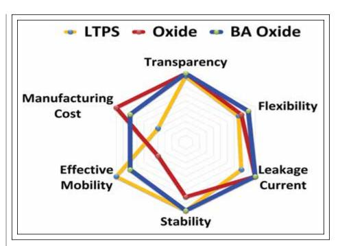
**Fig. 3:** The schematic illustrates a comparison among LTPS, oxide, and BA-oxide TFTs for flexible-display applications. The BA-TFT backplane has the advantages of manufacturing cost, flexibility, leakage current, and transparency compared to that of LTPS TFTs.
