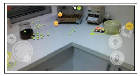
*Fig. 8:* The real physical world is augmented with virtually rendered 3D objects using a device with an embedded Intel RealSense module.<sup>10</sup> Here, a digitally rendered car is shown racing on a real table, with realistic physical effects such as collisions with real objects, correct occlusion and shadows, etc.
