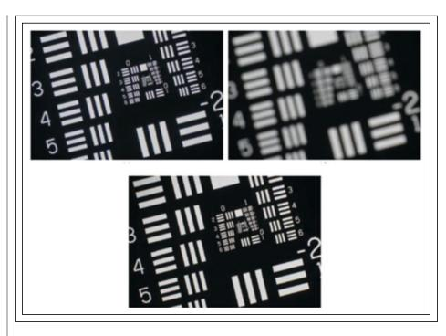
**Fig. 3:** Results from an adjustable liquid-crystal lens include a lens image taken with voltage applied to provide a 400-mm focal length to focus the image (top left), an LC lens image with 0 V applied (right), and a glass lens image with a 400-mm focal length for reference (bottom).<sup>5</sup>
