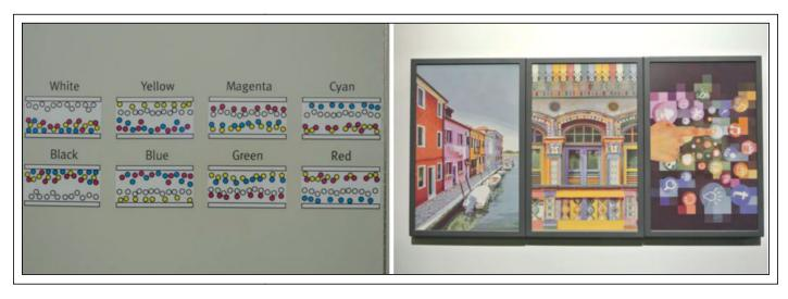
Fig. 1: E Ink's new color technology uses particles of four different colors within each microcapsule (left) that are controlled in such a way as to create thousands of colors for an unusually vibrant electrophoretic display (right).
