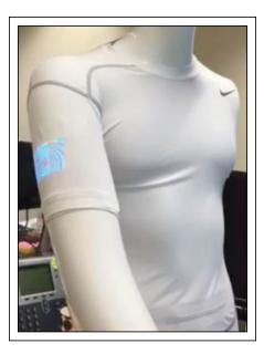
Fig. 2: This conformable  $64 \times 45$  RGB LED matrix is integrated into the sleeve of a t-shirt that is mounted on a mannequin. Source: IMEC, Ghent University, Holst/TNO, and Panasonic; 2016 SID Digest of Technical Papers.
