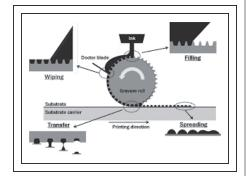
Fig. 1: In this conceptual view of gravure printing, ink is dispensed to fill wells in the gravure cylinder. Excess ink is wiped using a doctor blade. Ink is transferred to a passing substrate; the ink subsequently spreads and dries. Source: UC Berkeley; 2016 SID Digest of Technical Papers.
