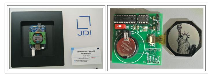
Figs. 5 and 6: At left, JDI's demonstrator was a 1.2-in. round MIP display. At right, Sharp's round 128 x 128 pixel display featured ultra-low power. Photo courtesy Jyrki Kimmel.
