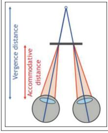
**Fig. 2:** The vergence–accommodation conflict arises from the difference between the point where the two eyes converge and the points to which the eyes focus or accommodate for traditional stereoscopic 3D displays.<sup>4</sup>
