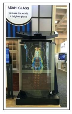
Fig. 2: This interactive virtual concierge robot is an example of Asahi Glass Co.'s Glascene technology, in which an image projected onto a transparent glass screen becomes an interactive presentation through motion sensing.
