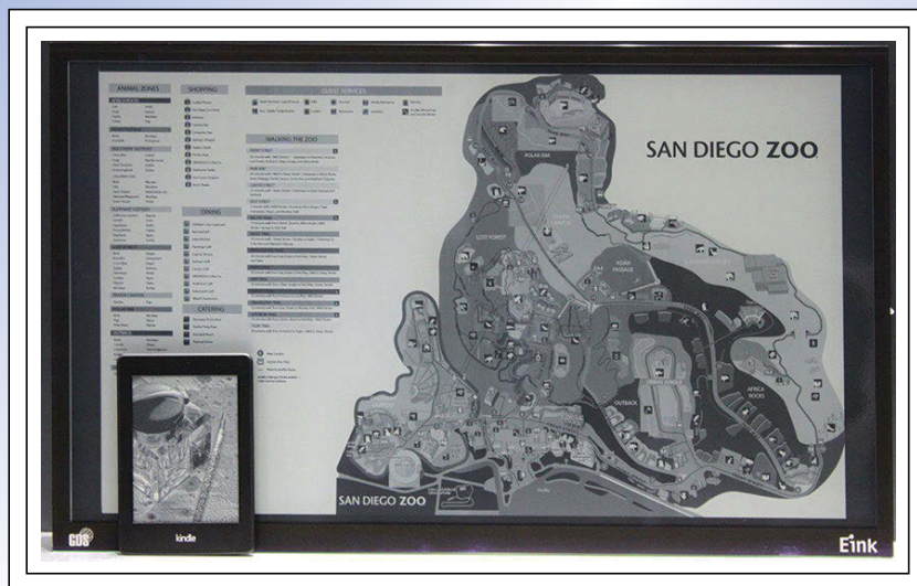
Fig.1: E Ink's new 32-in. electrophoretic display comes in gray scale (shown here) and color and is designed for indoor and outdoor signage.
