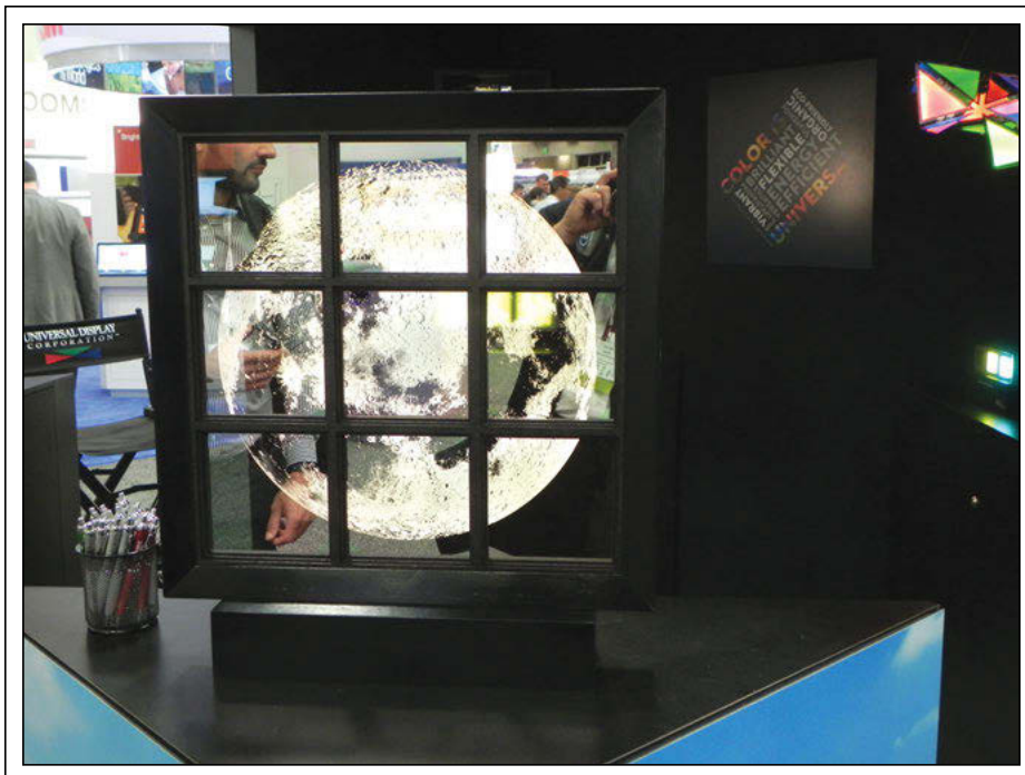
Fig. 5: Perhaps the most unusual display at the show was the Moon Window from Universal Display Corporation, which demonstrated how transparent white OLED panels can make windows a light source at night. Photo courtesy Alfred Poor.
