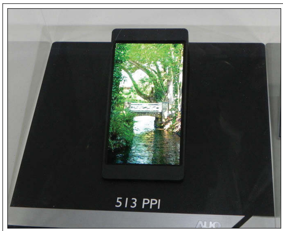
Fig. 1: AUO's 5-in. OLED panel has a pixel resolution of 2560 × 1440 for an impressive 513 ppi. It is rated at 300 cd/m 2 and produces imagery that looks almost as if it is printed on paper. Photo courtesy Alfred Poor.
