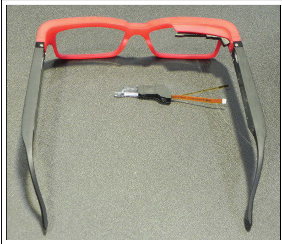
Fig. 4: Not all glasses are made by Google; the Kopin White Pupil demonstrator shows how Kopin's head-mounted display can be hidden in an eyeglass frame. Photo courtesy Alfred Poor.
