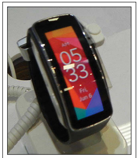
Fig. 3: The Samsung Gear Fit smart watch sports a curved OLED display that would be a lot more attractive if the rest of the watch were thinner. Photo courtesy Alfred Poor.
