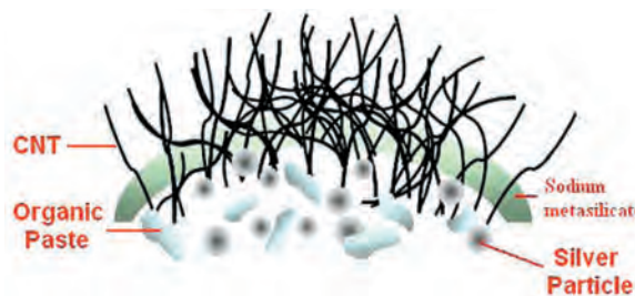
FIGURE 3 — Schematic diagram shows that the one end of the CNT is pulled by a magnetic force and bent upward.
