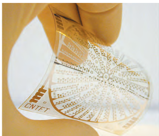
FIGURE 3 — Fully processed CNT-network TFTs on a 50 \times 50 \text{ mm}^2 PES substrate.
