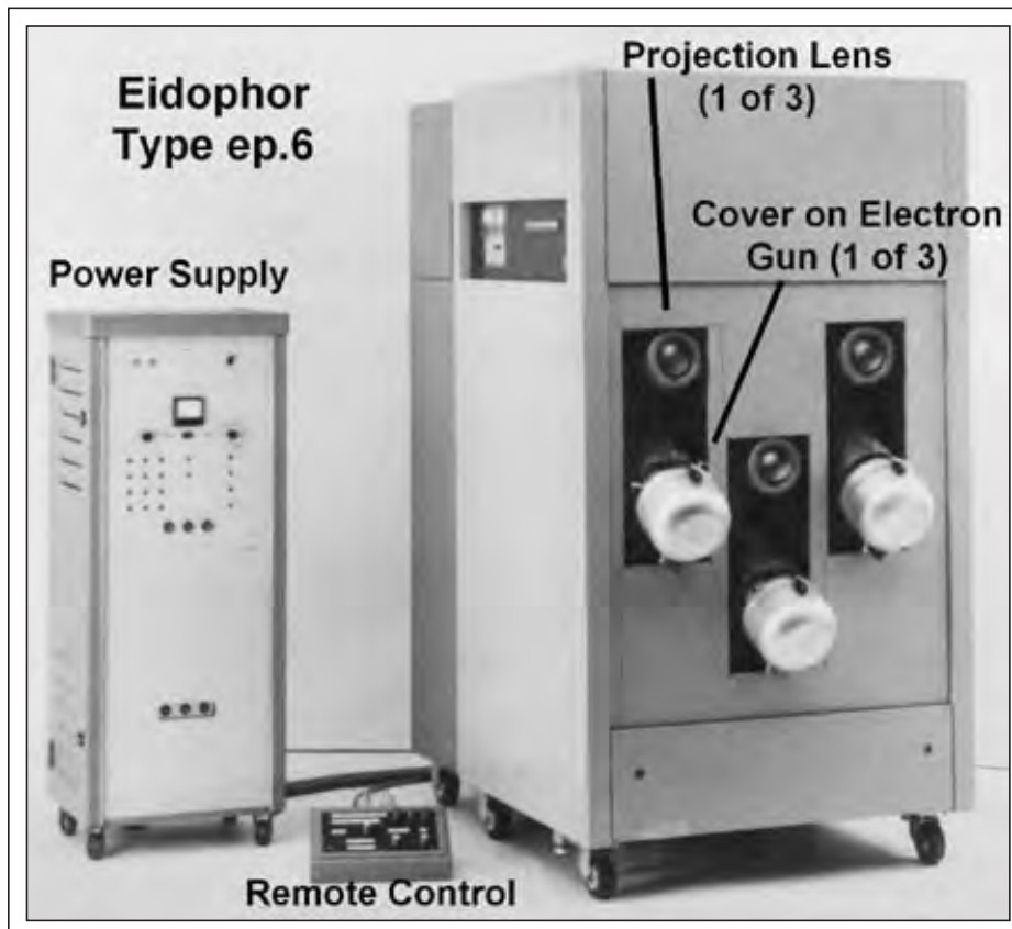
Fig. 5: Eidophor Model ep.6 simultaneous color projector capable of 2500 lum.
