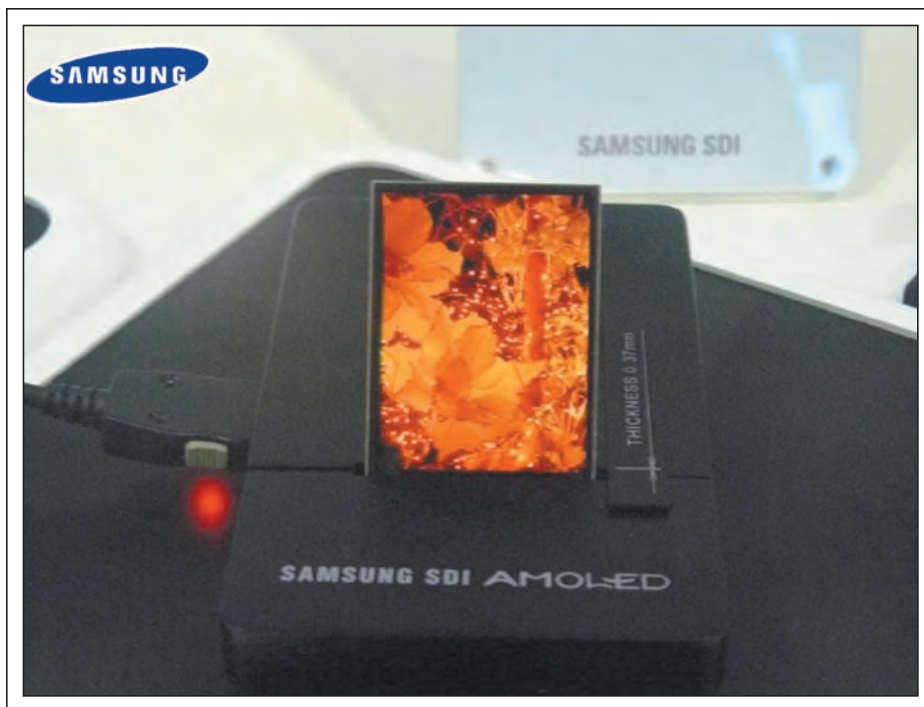
Fig. 1: The world's thinnest display made by Samsung SDI. A Vitex Barix coating is used as encapsulation.
