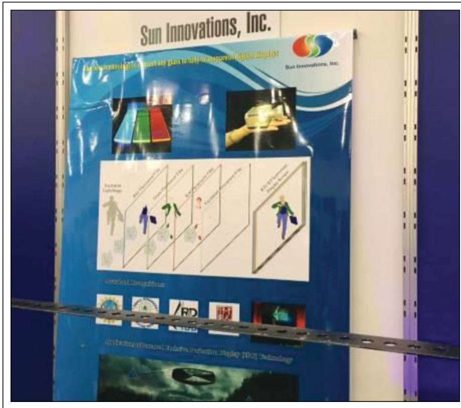
Fig. 5: Sun Innovations creates color-sensitive RGB films and excites them with a projector to create full-windshield HUDs.
