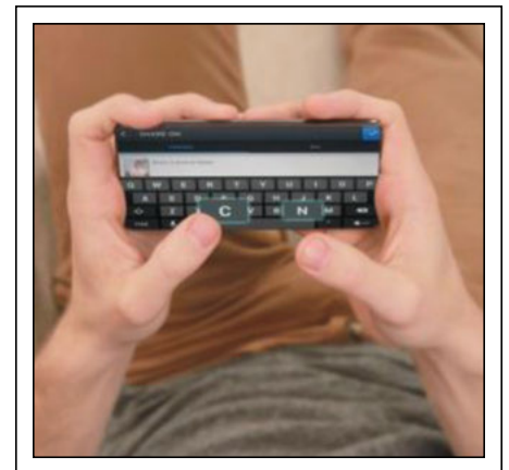
Fig. 5: Fogale Sensation's hovering technology allows accurate input without touch.
