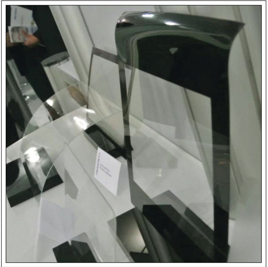
Fig. 1 Corning Gorilla Glass can be formed with a "local bend" for automotive applications. Photo courtesy Ken Werner.
