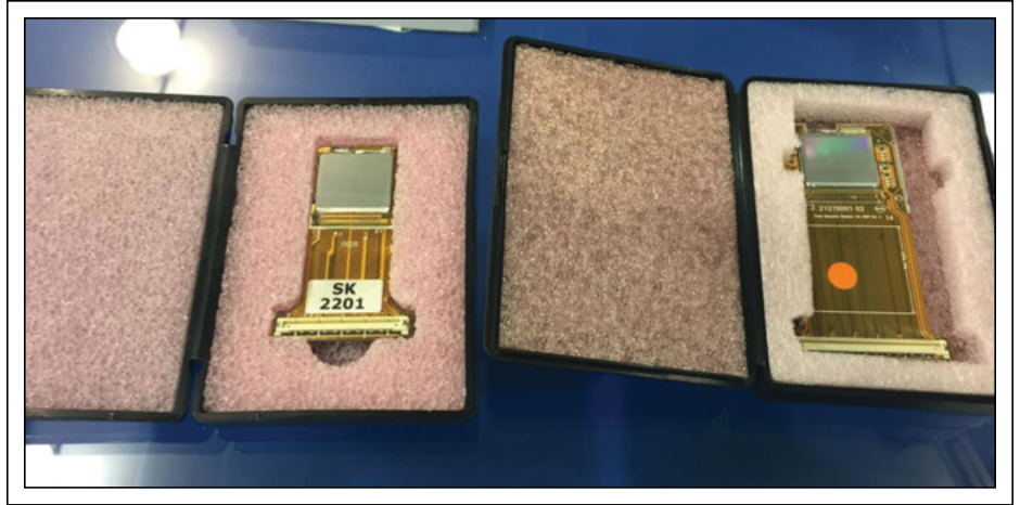
Fig. 2: These ForthDD high-resolution microdisplays shown at Display Week are now used in machine-vision projects well as high-end viewfinders.
