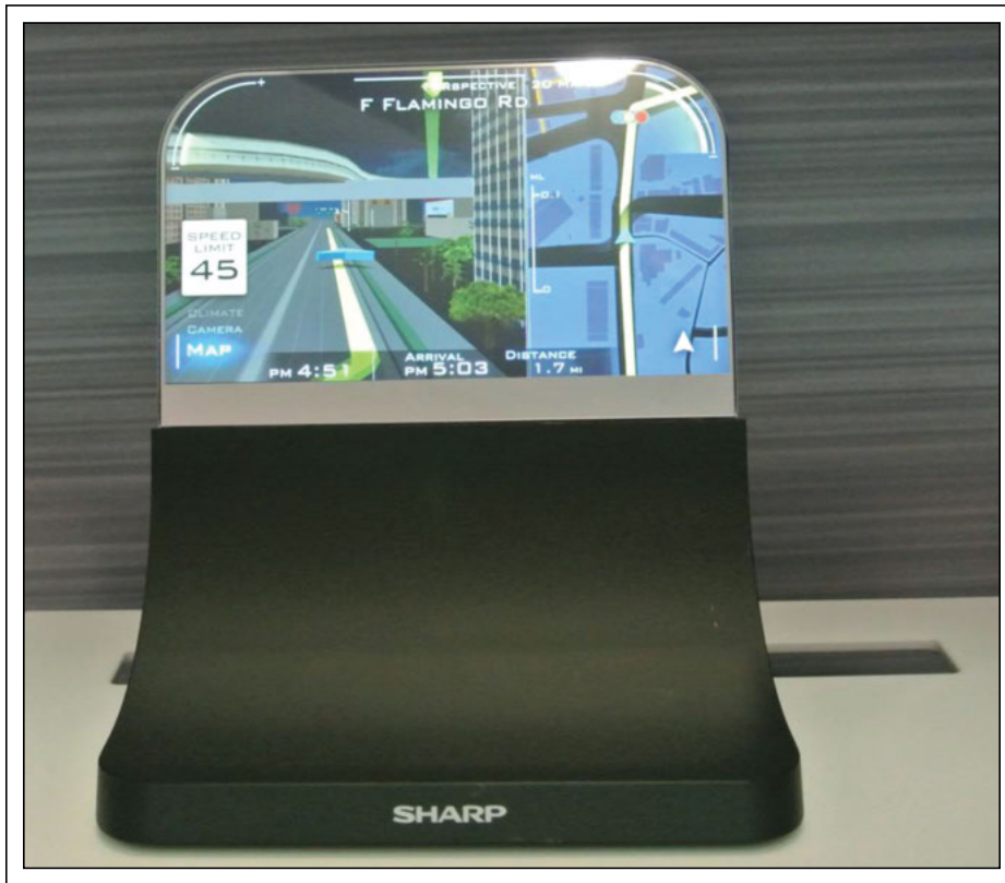
Fig. 4 This recent demo of Sharp's "free-form" LCD technology has a curved top and almost no bezel on the top three sides. The display incorporated touch on the outside edges of the display, not the surface. Photo courtesy Ken Werner.
