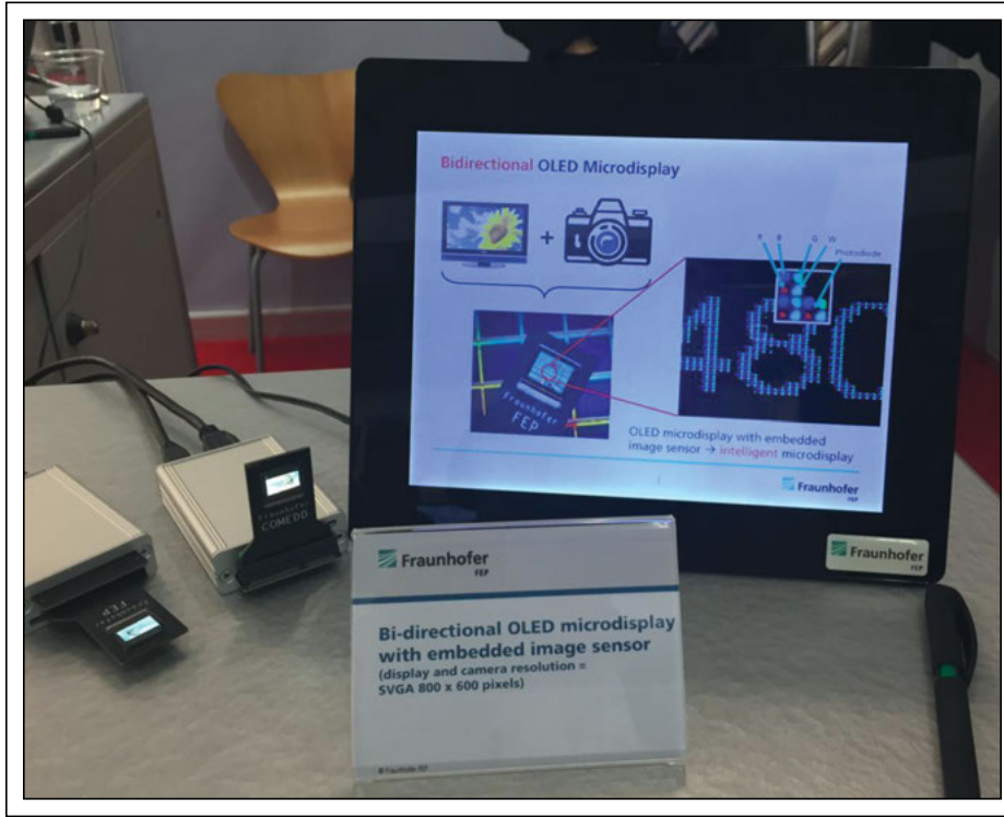
Fig. 3: Fraunhofer's bi-directional OLED microdisplay appears in the bottom left side of this image.
