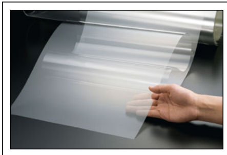
Fig. 4: Nippon Electric Glass's G-Leaf glass is less than 0.2 mm thick and, as a result, is extremely flexible.
