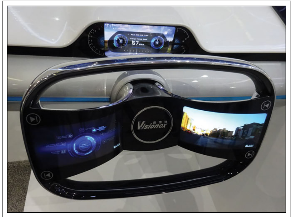
Fig. 3: In this demo steering wheel display from Visionox, the monitor on the right acts as a visualization of the rear-view camera, while the left display switches between operational data and touch control for an infotainment system. Photo: Karlheinz Blankenbach
