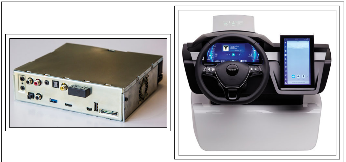
Fig. 4: On the left is the “silver box” for Visteon’s SmartCore controller and on the right, a demo of the interface for an upcoming generation of SmartCore. Source: Visteon.
