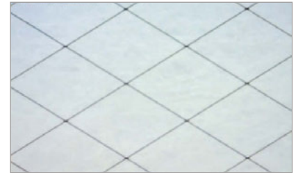
Imbedded Mesh ( \leq 5 OPS, T\% \geq 90\% @ 420-680nm)
