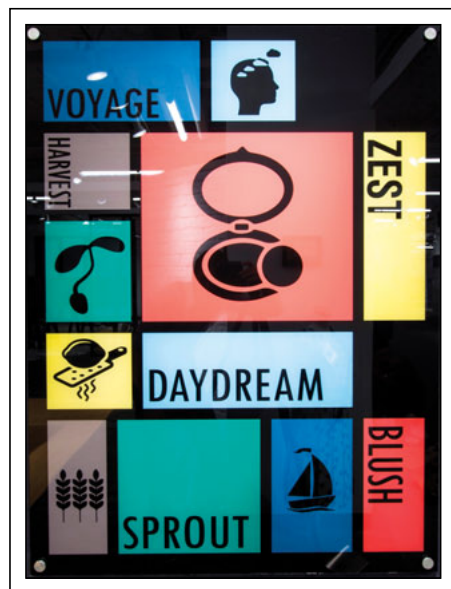
Fig. 1: The seven new colors available for E Ink Prism increase options for designers of low-power, reflective signage and architectural elements.
