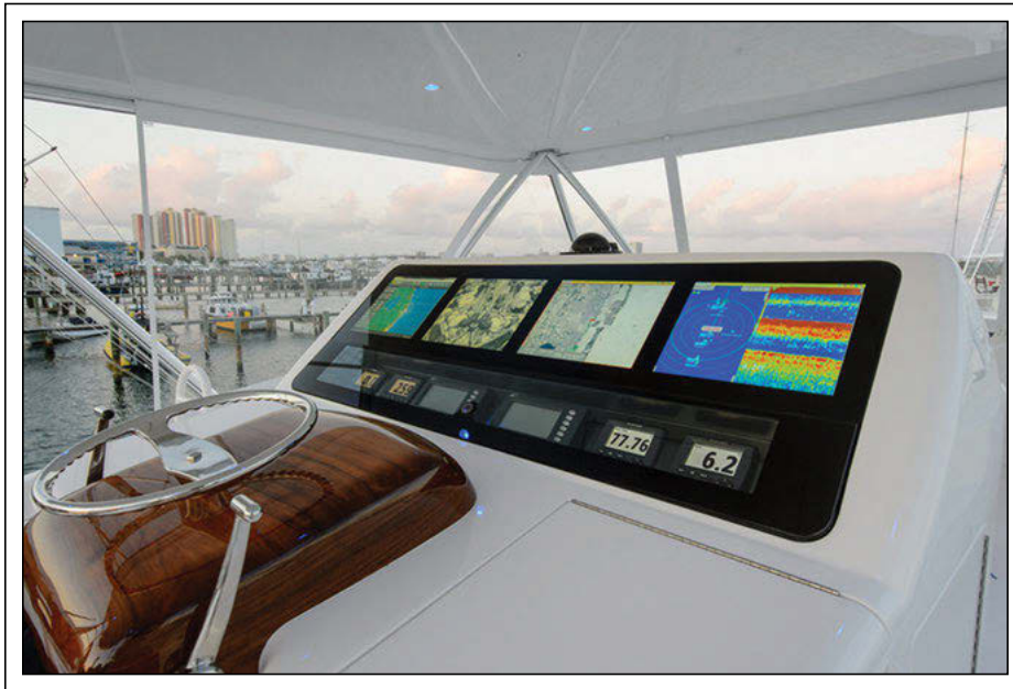
Fig. 4: Direct-dry-film bonding works well for combining multiple LCDs on one sheet of large glass, as is often desired in luxury yachts. Image courtesy Kessler–Ellis Products.
