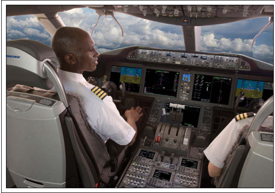
Fig. 3: A variety of dry-film optical bonded displays are used together in this cockpit. Image courtesy Boeing.
