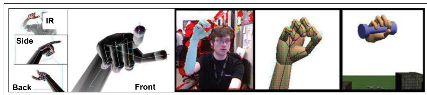
Fig. 5: An articulated model-based hand-skeletal tracking technology enables fine-grain versatile manipulation of objects in 3-D space. Source: Intel.
