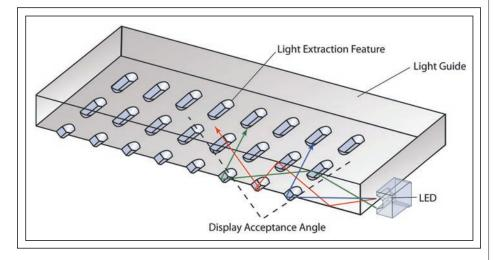
*Fig. 4:* In many touch-enabled display graphics applications, one LED can be used to illuminate multiple graphic icons.
