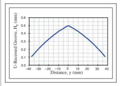
Fig. 4: The height of the "U-groove" increases along the y-axis in order to decrease the leakage of the light to the neighboring segments. The increase of the groove's height is the same as the left side groove. The peak of the graph shows the center of the LGP.
