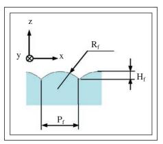
*Fig. 6:* The light-cone-shaping feature is shown on the LGP. This is an array of low-power light-collimating lenses.
