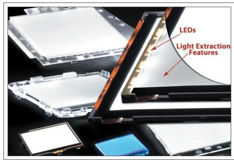
**Fig. 2:** LEDs positioned on the edge of the light guide employ pixel-based light-extraction features. As shown in the background, mechanical holding features can be designed into the backlight.
