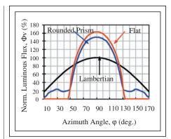
Fig. 2: The light distributions are shown inside and outside of the LGP. The LED distribution has a semi-Lambertian luminous distribution. The distribution is widened after passing through the light-injection features. For comparison, the light distribution after passing a flat light injection surface is plotted.
