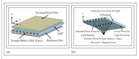
**Fig. 1:** (a) Left: the structure of a monolithic BLU. The BLU is a combination of a functional LGP, 16 pseudo-white LEDs, a LGP reflector film, and an inverted prism. (b) Right: An LGP with light-controlling features on the light injection surface, back surface, and "V-groove" optical partition.
