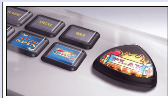
INCOM's fiber-optic technology enables keypad keys whose displays are changeable through programming just one LCD panel. Photo courtesy INCOM.
