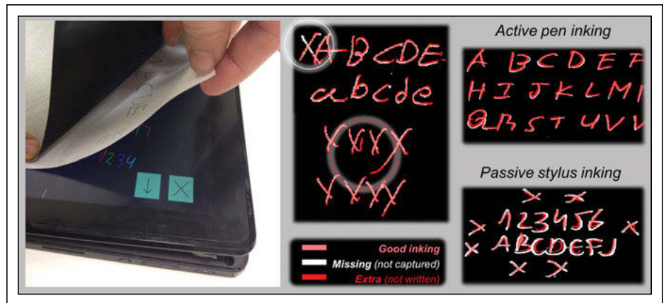
Fig. 9: At left, an inking test uses carbon copy and paper placed over a display as a reference for digital writing. The center example shows good inking in pink, missing strokes in white, and extra strokes in red. At right, active and passive stylus inking is compared.
