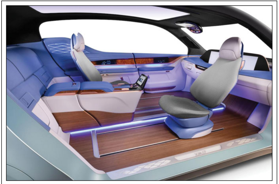
Fig. 2: The XiM17 interior concept from Yanfeng Automotive Interiors demonstrates several potential uses of curved displays, including a door-panel display and a floor-console display. 3 Yanfeng is actively sourcing conformable display technologies from a number of sources to make this concept a reality. Image: Yanfeng Automotive Interiors
