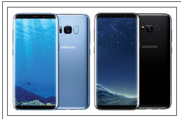
Fig. 1: Samsung's new 5.8-in. Galaxy S8 (left) and 6.2-in. Galaxy S8+ (right) feature displays that cover nearly the entire front face of the phone. The Galaxy S8 has a 570-ppi display, and the Galaxy S8+ has a 529-ppi display. Photos: Samsung
