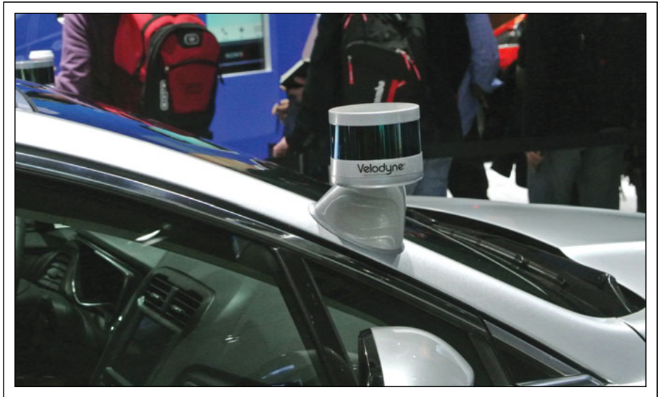
Fig. 3: A Velodyne lidar sensor is mounted on a developmental Ford vehicle. Lidar is regarded as an essential technology for autonomous vehicles. Ford recently announced it would field Level 5 autonomous vehicles in 2021. Photo: Ken Werner
