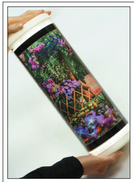
Fig. 4: FlexEnable's plastic organic LCD (OLCD) is shown here in a cylinder form factor. OLCD displays can be curved to bend radii of below 30 mm.
