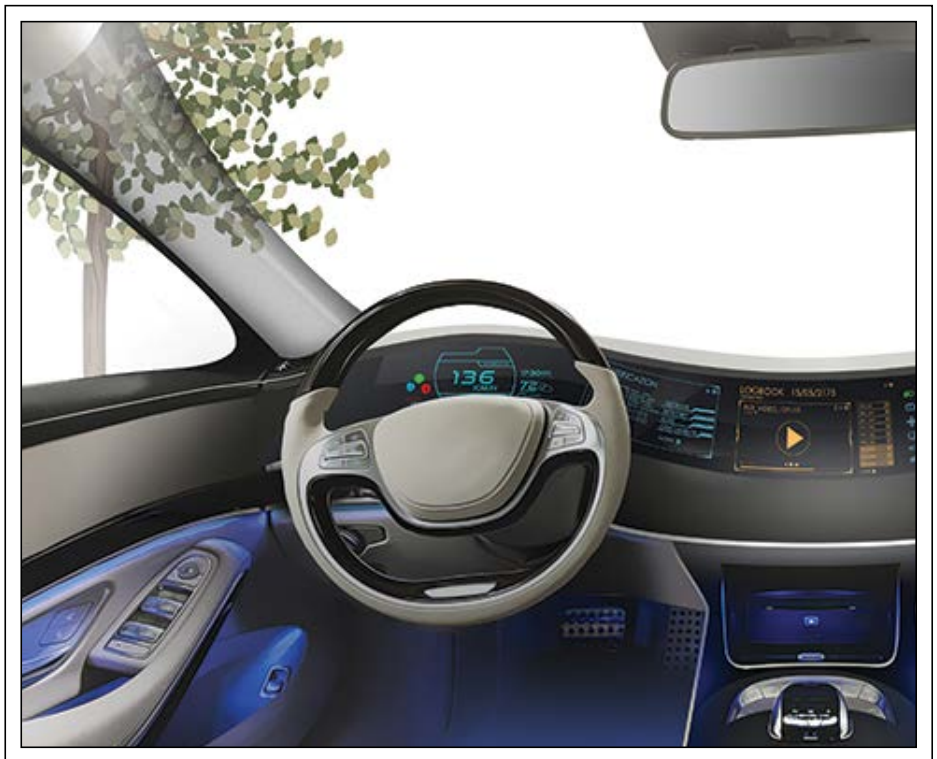
Fig. 1: The transparent pillar concept is illustrated here. The supporting pillar on the left next to the windshield appears transparent to the driver, revealing potential road hazards. This is enabled by a conformed wrap-around display that is projecting an image from an external camera. Image: FlexEnable
