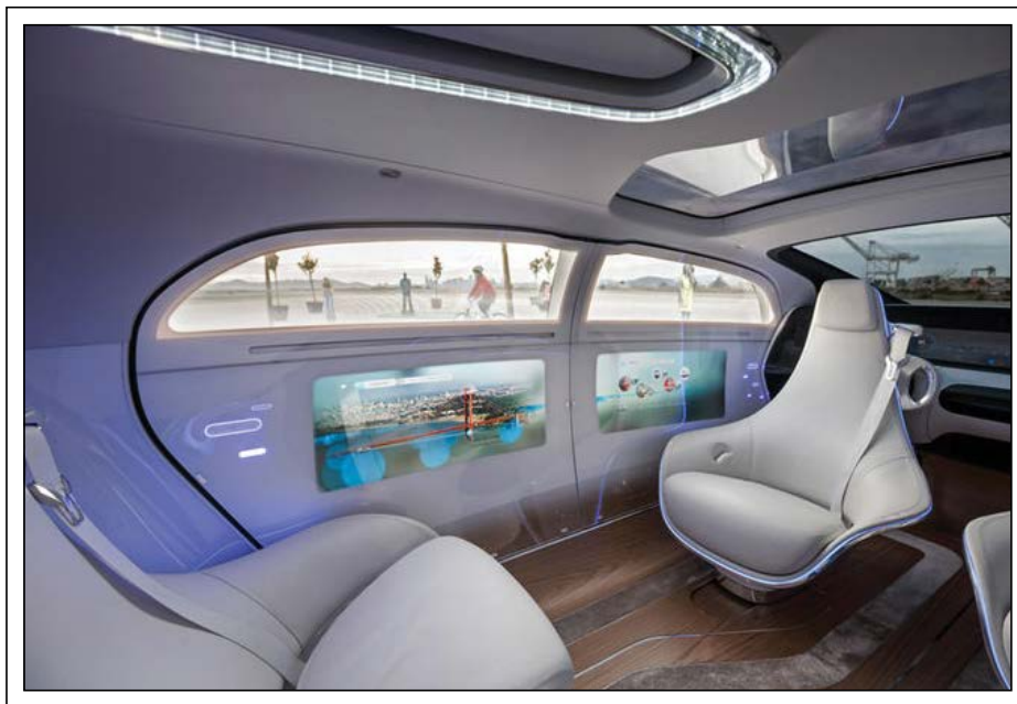
Fig. 4: When the car drives itself, what do you do? You might want to watch the multiple wide-aspect-ratio door-mounted displays. Photo: Daimler Benz
