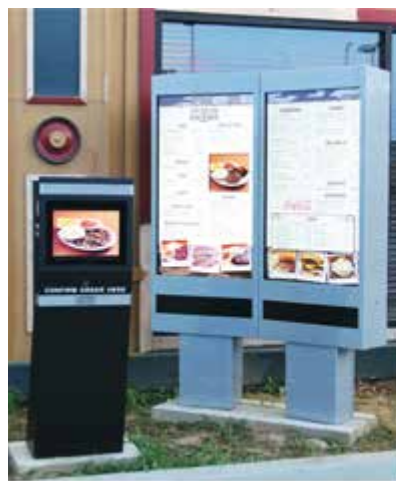
Fig. 1: These outdoor LCDs (with some key features listed above) are used for a restaurant drive-thru menu and order confirmation application.
