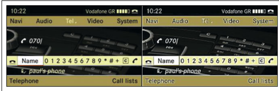
Fig. 12: Sunlight optimization of UI content appears above with an edge enhancement filter applied to gain readability of the UI content.
