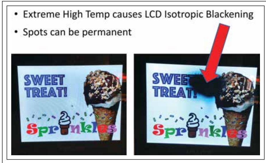
Fig. 2: The liquid-crystal mixture in the LCD at right has suffered from isotropic blackening effects, which can occur as a result of high temperatures.
