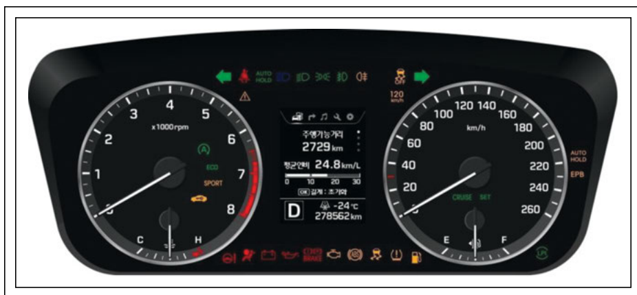
Fig. 1: This instrument-cluster meter with a 3.5-in. PMOLED display (center section of display) manufactured by DENSO for the Hyundai Sonata shows seamless integration of the display, with no display outline and no different background since the contrast ratio is more than 100,000 to 1.
