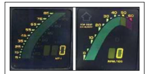
Fig. 2: The first digital speed and tachometer LCDs, by Hitachi and Delco, appeared in the 1984 Corvette. Image courtesy Bob Bordo, GM.
