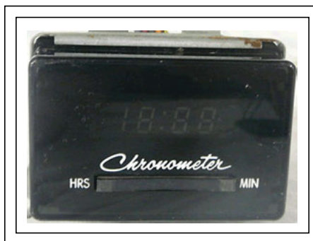
Fig. 1: The first digital clock in an American automobile was a vacuum-fluorescent display from Futaba, in the 1976 Dodge Aspen. Image courtesy Ben DiCicco/Chrysler.
