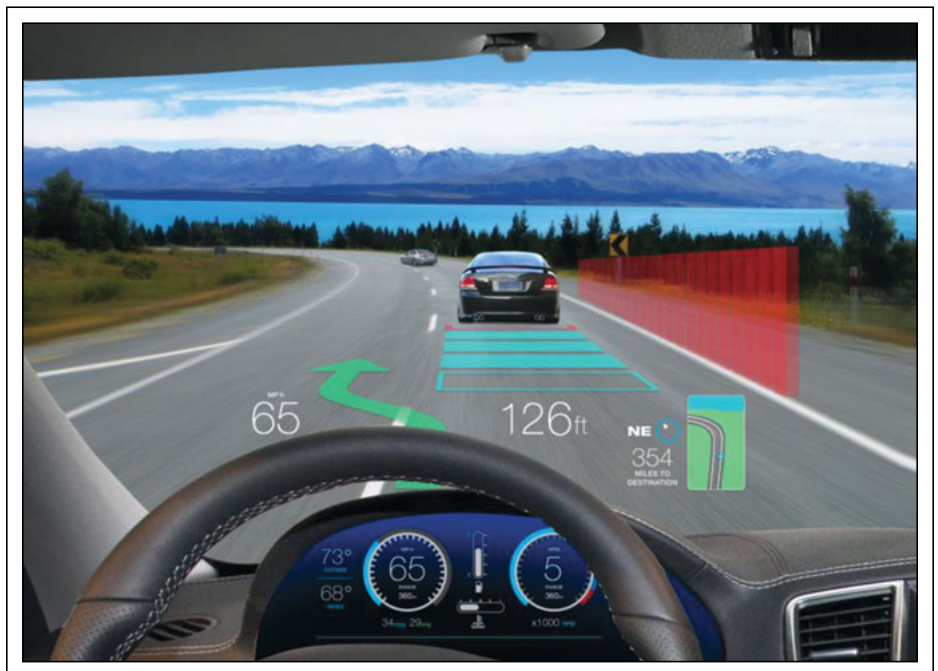
Fig. 1: An augmented-reality HUD shows conformal graphics over the driver’s line of sight.
