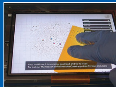
Fig. 3: Tianma's new 8.4-in. XGA TFT-LCD provides dry screen tracking, water build-up tracking, and single-glove operation, even in a wet environment. It can also be used with medical-grade defibrillator gel and ultrasound gel.
