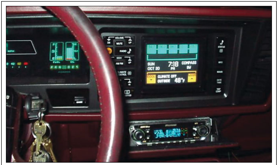
Fig. 3: The first automotive digital information center with a touch screen was introduced in the Oldsmobile Toronado in 1989. It featured a color CRT display with infrared touch by Denso. Monocolor for the Buick Riviera by Delphi.
