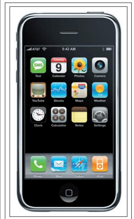
Fig.1: The use of multi-touch in the iPhone fired the public imagination and helped bring about general acceptance of the multi-touch interface. Image courtesy AT&T.
