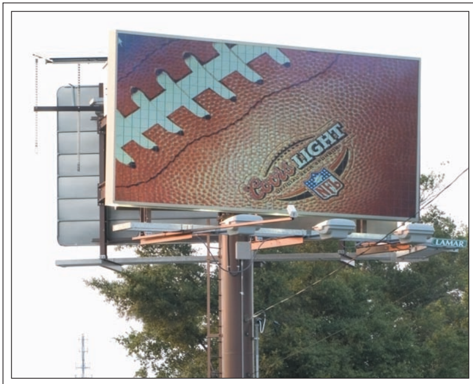
Fig. 3: Shown is a 20-m 2 high-contrast ChLCD from Pensacola, Florida, 2008.
