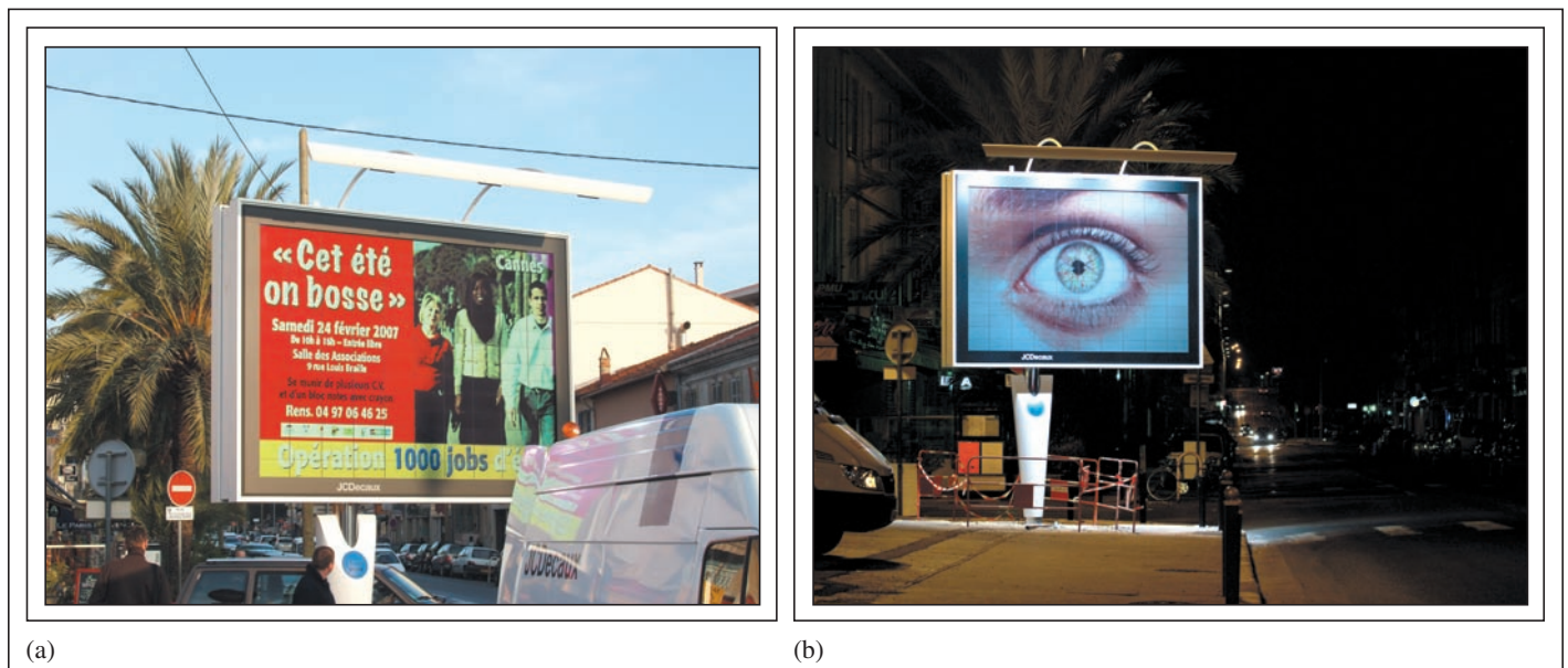
Fig. 2: Shown is a 6\text{-m}^2 high-contrast ChLCD – (a) day and (b) night views – erected in Cannes, France, in 2006.
