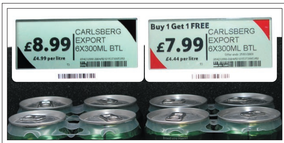
Fig. 4: Some of the ZBD options shown at SID's Display Week 2008 included the use of area color (top left shows the display with black corners and top right with the same display and the corners latched to red).
