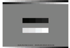
Figure 1. Pattern (SET01S50) to set up the front-projector.
