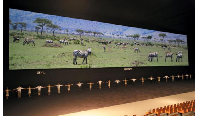
FIGURE 1 — The GLV laser projector demonstrated at 2005 World Exposition, held in Aichi, Japan. The screen size is 50 × 10 m. Twelve 5000-lm laser projectors were used.
