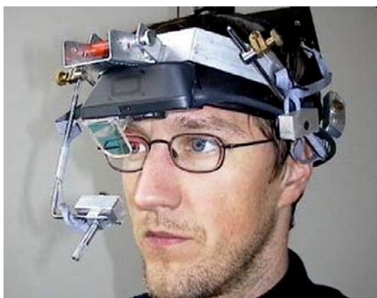
FIGURE 3 — Mock-up system consisting of a microdisplay and a head-mounted eye-tracker simulating the bi-directional see-through HMD.
