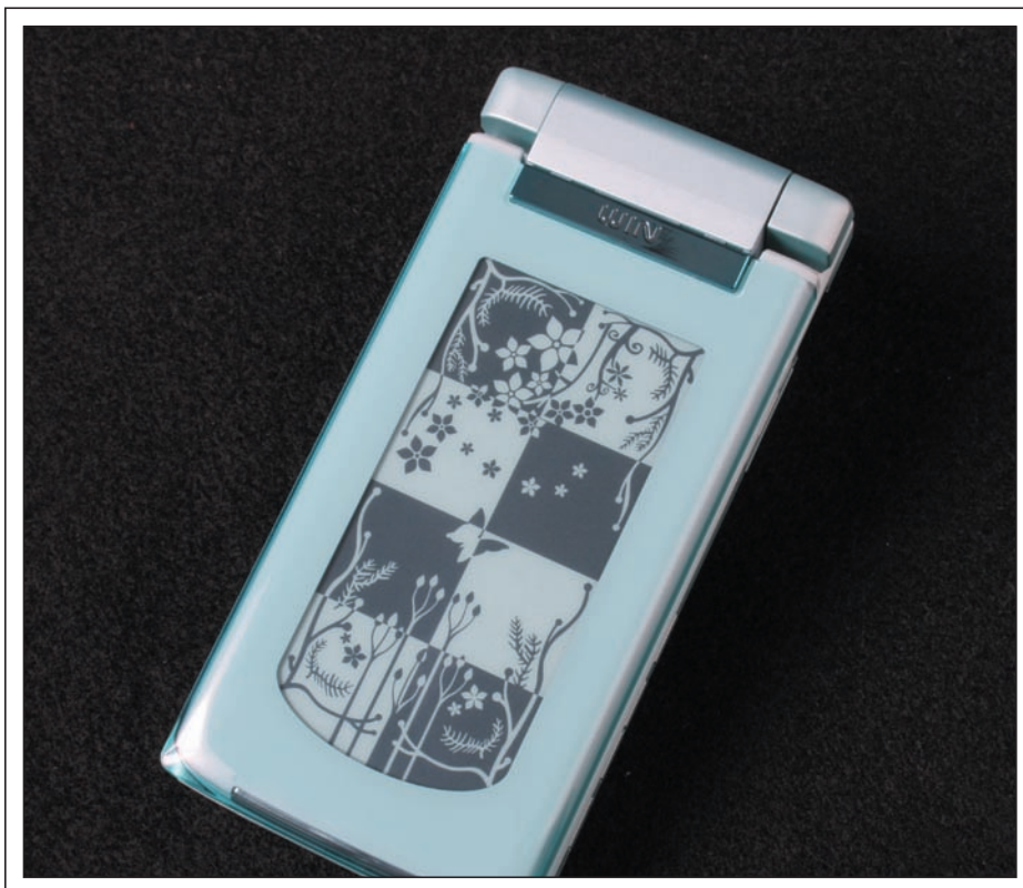
An Hitachi mobile phone features a flexible display from E Ink on its cover. Image courtesy of E Ink.
