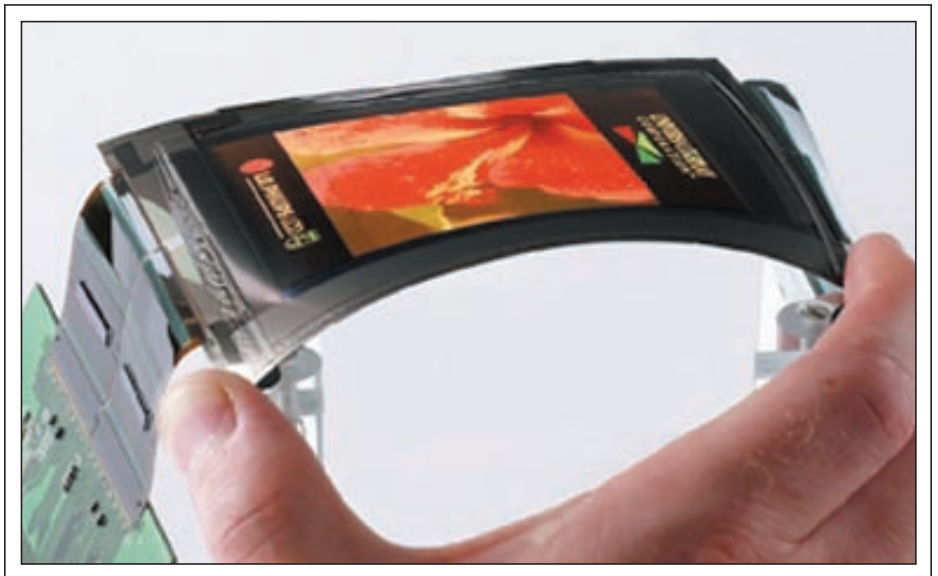
A flexible OLED display developed by Universal Display Corp. and LG Display represents just one of the technologies currently under development for potential military and commercial applications. Image courtesy of UDC.
