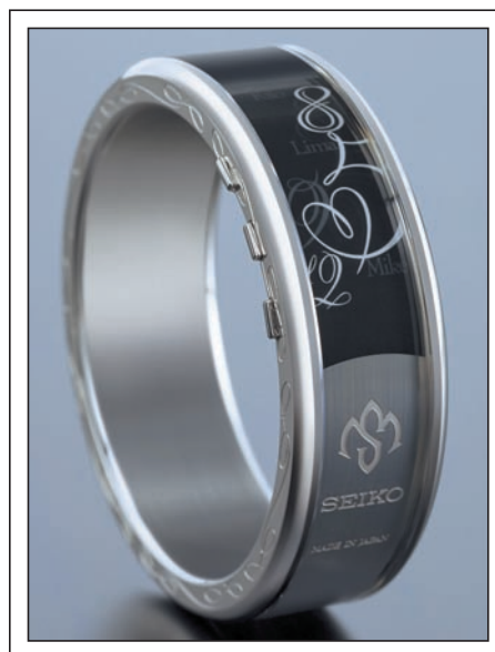
Fig. 1: EPDs, custom IC drivers, and low-power MCUs made it possible to create an innovative design for Seiko's bracelet-style wristwatch for women. The black-and-white display runs along the exterior of the band and is capable of displaying the time in "efficiency" mode with easily recognizable numerals or in high-concept "mystery mode," as shown here. In mystery mode, the numerals appear in script in somewhat mysterious patterns. For example, the time shown here is 12:58, reading from the lower left-hand side of the display upwards (the "1" is only partially visible at the left) and right to the "8". Image courtesy of Epson.
