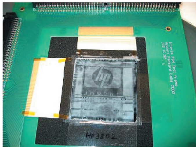
FIGURE 10 — Plastic version of 85-dpi 100 \times 100 passive-matrix-addressed EPLC display with black dyed LC and white pigments, controlled by a 40-V electrical driver.
