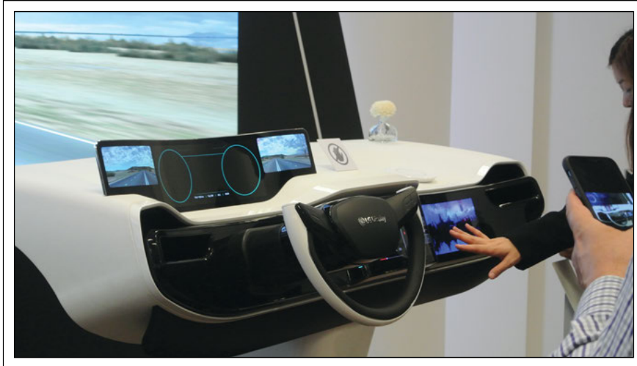
Fig. 5: This LG Display cockpit concept is notable for the nice integration of the various displays and the positioning of the side-view images on the same display as the instrument cluster. (Photo: Ken Werner)
