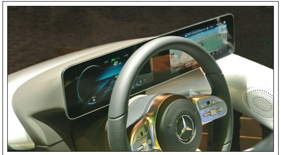
Fig. 4: The Mercedes-Benz MBUX offers a wide-screen display that is both modern and modest, which is appropriate for its intended application in M-B's new generation of compact A-Class cars. (Photo: Ken Werner)
