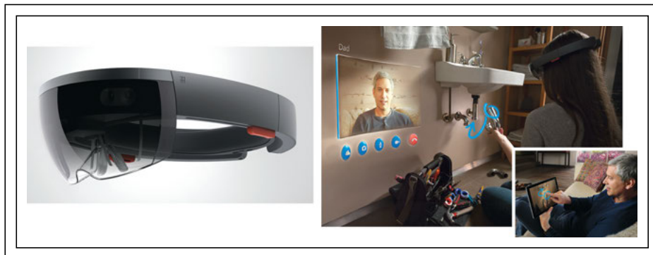
Fig. 2: A popular AR device (which its maker refers to as a mixed-reality device) is the HoloLens from Microsoft. The headset at left enables augmented-reality applications, including remote plumbing repairs, as shown at right. Source: Microsoft
