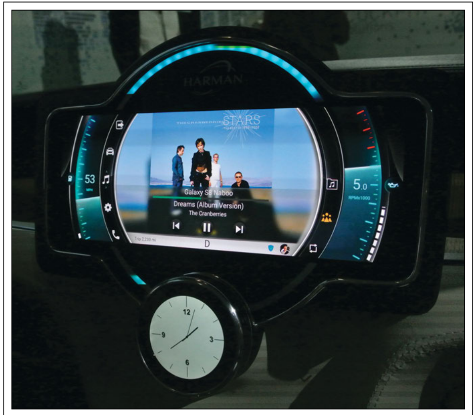
Fig. 2: Harman designed this demonstration QLED cluster for the MINI dashboard to combine instrumentation (in the outer ring) and infotainment in the center. The user can change the infotainment part of the display but not the instrumentation part. The secondary display, showing a clock in the photo, changes content as the outside ring is turned. (Photo: Ken Werner)
