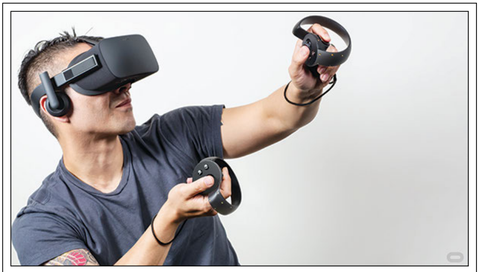
Fig. 1: The Oculus Rift is a well-known VR headset that enables users to experience immersive applications in which they see nothing of their physical surroundings. Source: Oculus
