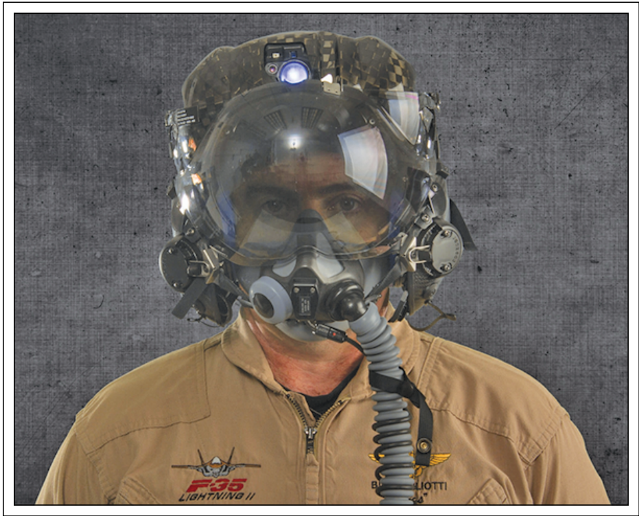
Fig. 7: The F-35 Lightning II helmet offers powerful AR capabilities but isn’t feasible for the consumer marketplace. Source: Lockheed Martin
