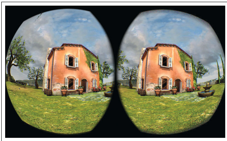
Fig. 5: Stereoscopic systems show two images to users. The images converge to create the perception of depth. Source: Oculus
