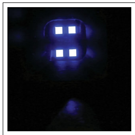
Fig. 1: Above are four true QLED subpixels as demonstrated by Nanosys. The subpixels are blue, but so bright they appear white even with the camera's exposure compensation set to maximum underexposure. Photo courtesy Ken Werner.
