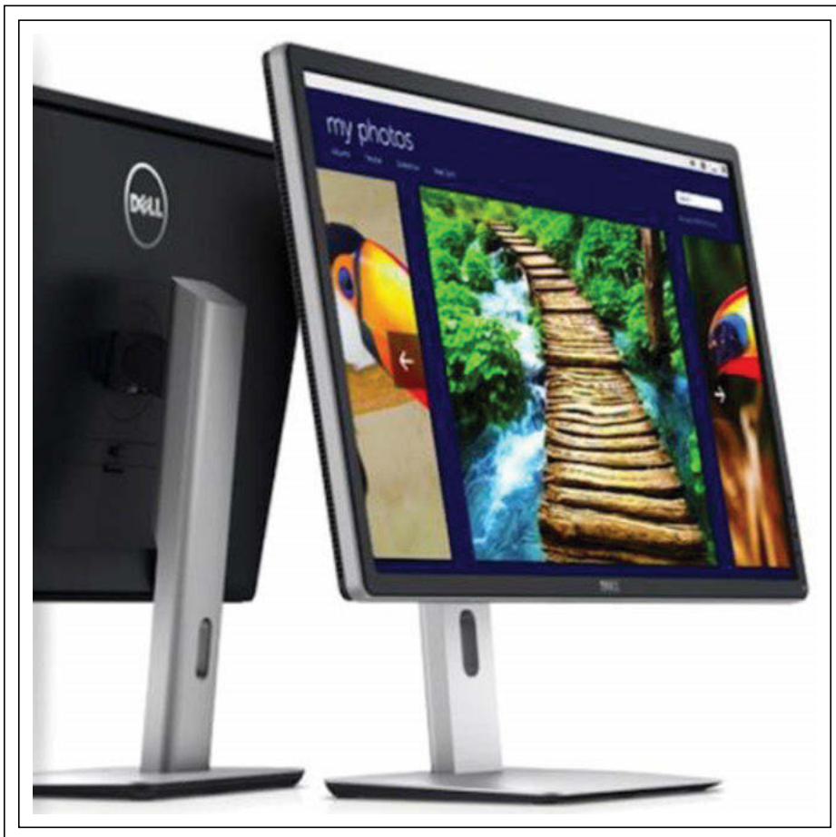
Fig. 3: Dell’s new low-cost 28-in.-diagonal UHD monitor with a TN-LCD was scheduled to start selling in Q1 for just $699, with 1.07 billion colors, 170° viewing angle, and 5-msec response time. Source: Forbsimg.com.
