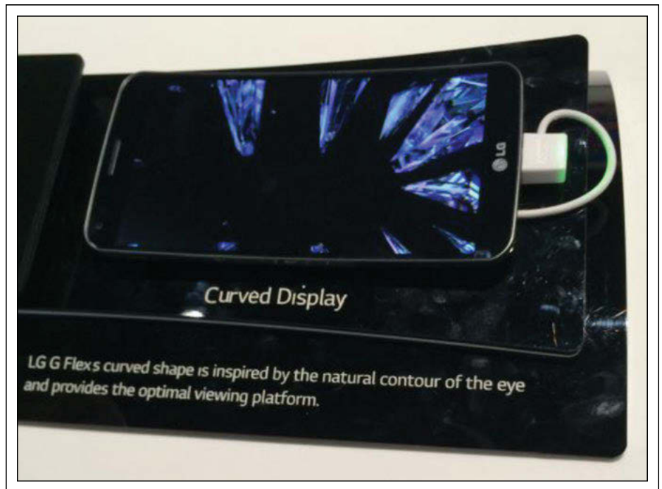
Fig. 2: The LG G Flex Smartphone with 6-in. curved POLED Display has a “self-healing” back cover. Photo courtesy Sechrist 2014.
