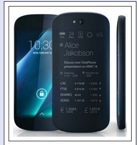
Fig. 2: The two-sided Yotaphone features a monochrome touch e-paper display on one side and a colorful AMOLED display on the other.
