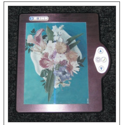
Fig. 3: E Ink Vizplex color displays will employ an RGBW color filter. Image courtesy E Ink.
