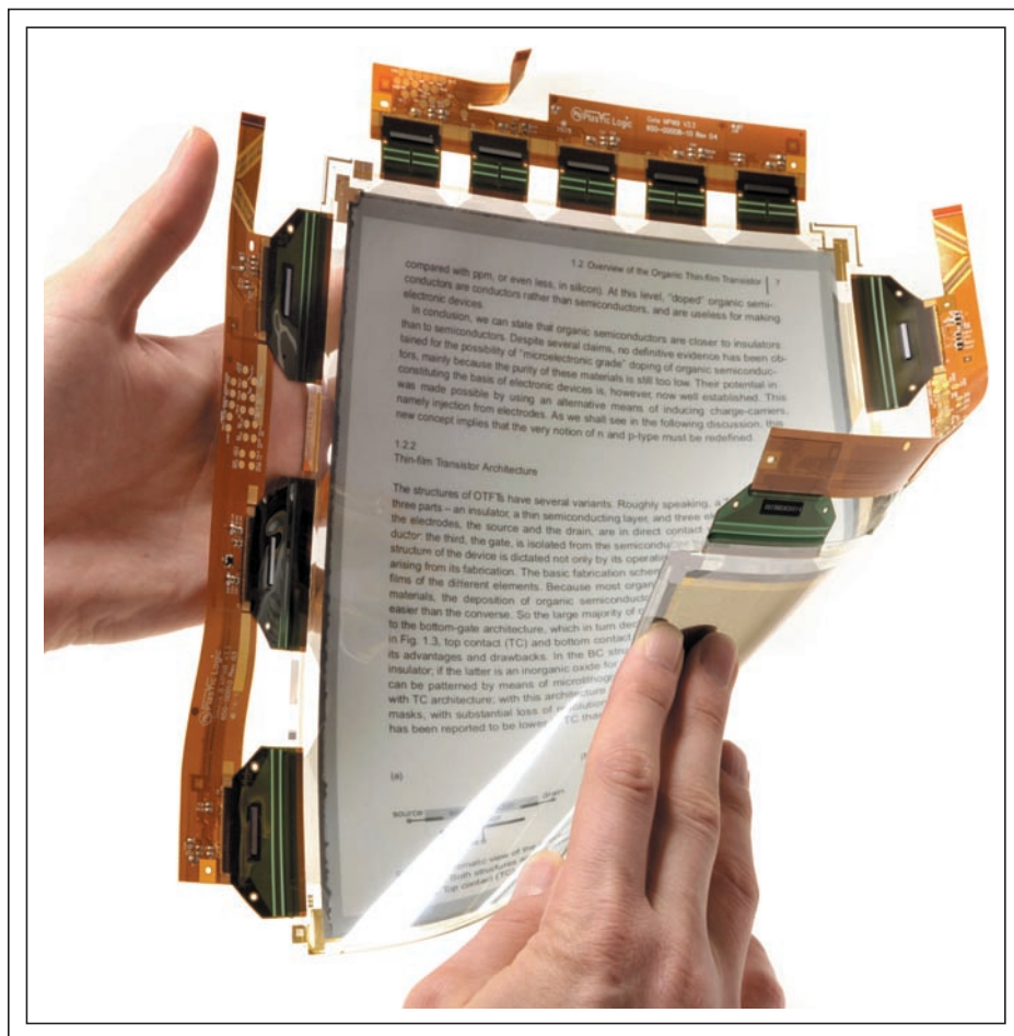
Fig. 2: This flexible display module made with plastic electronics in the Dresden facility in late 2009 has a resolution of 1280 \times 960 and 150 \text{ ppi} . The display media is Vizplex provided by E Ink Corp.
