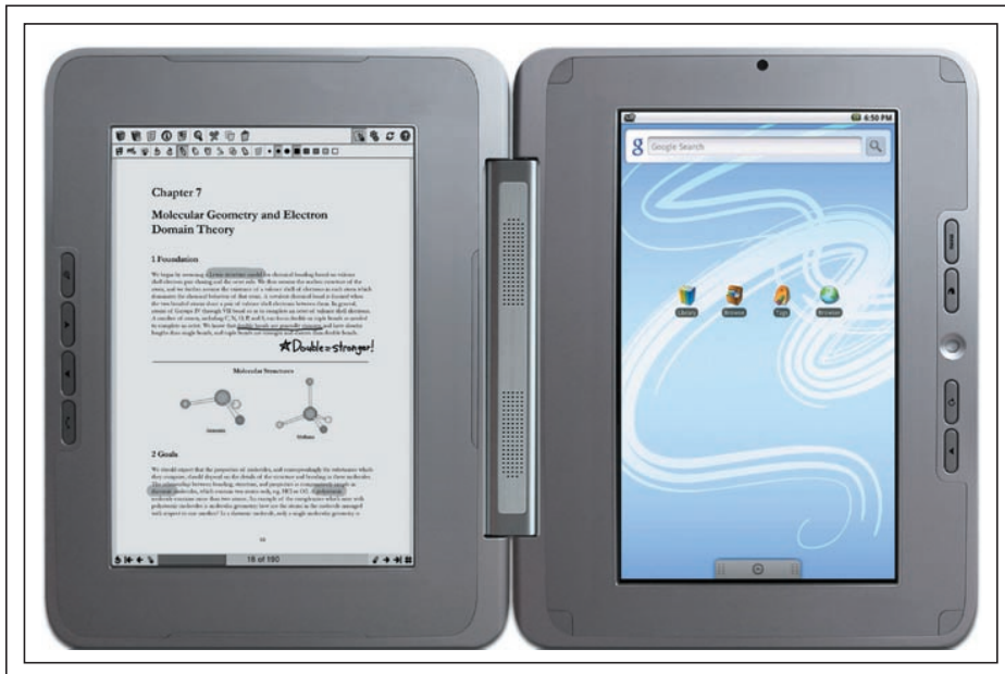
Fig. 4: The eDGe reader, which maker Entourage Systems calls a “dualbook,” features a 9.7-in. E-Ink-based screen on the left and a 10.1-in. LCD touch screen on the right. Users can call up a virtual keyboard for typing. It weighs about 3 pounds and is scheduled to ship in March 2010 at a cost of $490. Image courtesy Entourage Systems.
