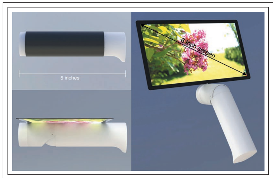
Fig. 7: A camcorder concept with a flexible AMOLED screen (designed by Emory Krall from Universal Display Corp.).
