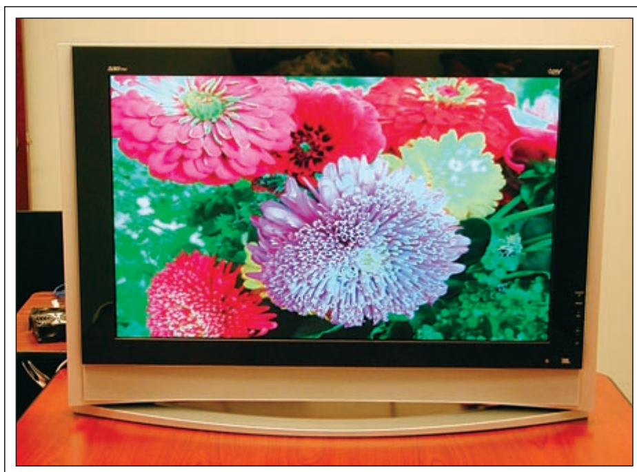
Fig. 1: One of the first edge-lit LED-backlit LCD TVs was this 32-in. version shown at the 2005 SID International Symposium in Boston. Today, this sized LCD can be backlit by as few as six RGB LEDs.
