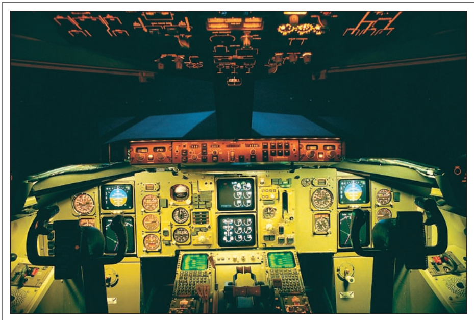
Fig. 4: In darkness, the levels of instrument, control, and interior lighting must be balanced to maintain the pilots' night vision, yet still ensure that all information sources are readily visible.
