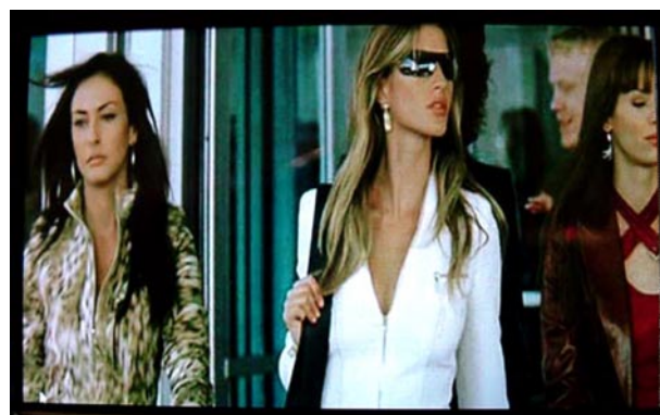
FIGURE 8 — 3.0-in. 308-ppi WVGA AMOLED prototype panel using a top-emission white OLED with color filters.
