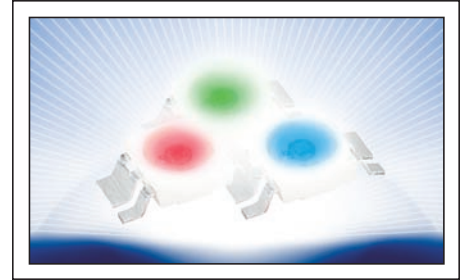
Fig. 3: Advanced Power TOPLED Plus LEDs have a low profile – 2.25 mm high – that enables the design and production of very thin backlights.
