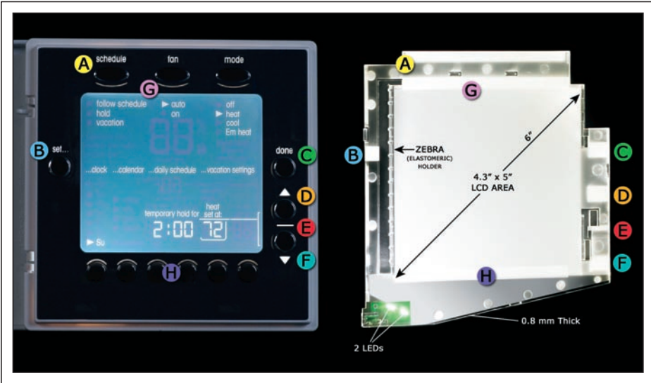
Fig. 3: This light guide lights nine discrete areas of this thermostat: the main LCD area, characters and directional symbols at the top and sides of the unit (A-F), and keypad buttons with “halo” effect at the top and bottom (G and H).
