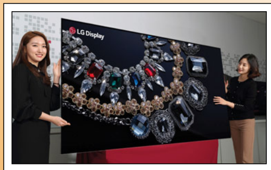
Fig. 3: LG Display's new 88-in. 8K OLED display incorporates 33 million pixels.
