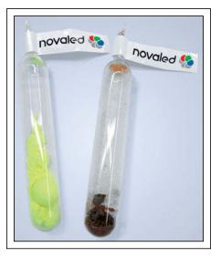
**Fig. 3:** The ampoule on the left shows the SoA ETL material measured after exposure at 318°C and the one at right, the same material after exposure at 368°C.
