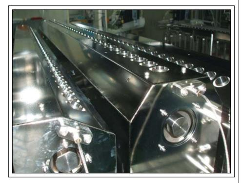
Fig. 2: This linear-nozzle-source deposition equipment is from Sunic Systems in Korea.
