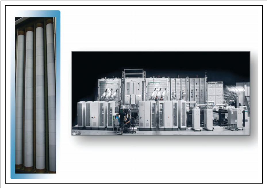
Fig. 1: This rotary target array consists of 12 Gen 8.5 IGZO sputter targets (a subset is pictured at left) installed in an Applied Materials PIVOT ® -sputtering system. (For a sense of scale, note the person standing in front of the system.) Image courtesy Applied Materials, Inc.
