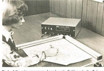
Each of the microprocessor-based sonic digitizers in the Science Accessories' GP-6 series are now available with optional 0.005' resolution for use in high-precision applications. The option provides up to 500 measured points per inch, compared to the standard 100 points per inch, 0.01" resolution.
