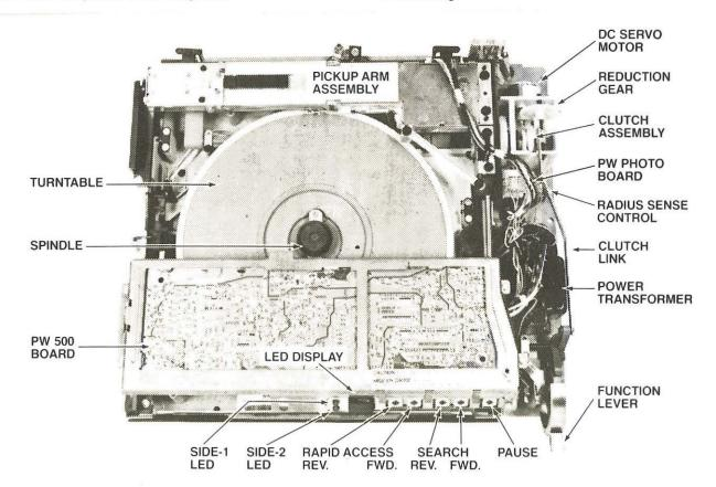
Figure 9. Top View of VideoDisc Player with Case Removed.
