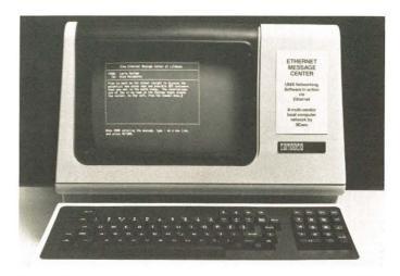
One of the Comdex Ethernet message stations consists of a DEC VT103 terminal with a plug-in LSI-11 processor. It is also equipped with 3Com's new Q-bus Ethernet controller and UNET software running with the Xenix operating system.
