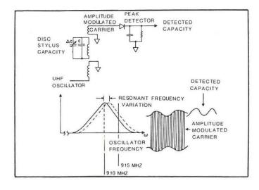
Figure 4. Close-up of Stylus Pickup.
