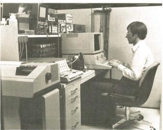
New HP 983A desktop computer, with 12-inch CRT screen, the availabilty of Pascal, and dual 51/4 inch flexible disc drives, is designed specifically with computer-aided engineering and computer-aided test applications in mind.
