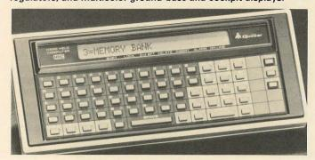
Hand-held computer from Quasar Company, Franklin Park, IL, features a 6502 microprocessor, and is programmable in Microsoftrm Basic and SNAP, a FORTH-like language. Optional peripherals connect the computer to large mainframes and databases over telephone lines, and to a conventional television receiver for local display. A thermal printer, RS 232C interface, and extra memory are also available.
