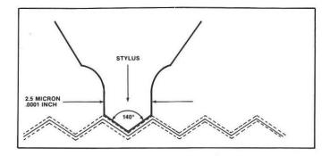
Figure 3. Disc and Stylus Cross Section.
