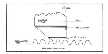
Figure 5. Signal Pickup.
