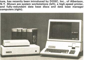
Enhanced by seven application software packages, an upgraded operating system and a 5-megabyte mass-storage system, the Apple III is an computer designed for professional end users as well as OEMs and systems integrators, the maker states.
