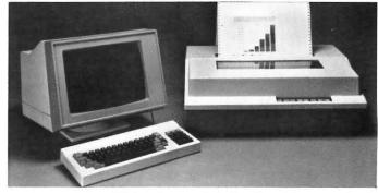
The Envision 230 Advanced Color Graphics terminal incorporates high-level graphics features useful for advanced business and engineering applications. In addition to a full range of scaling, rotating, and area fill features, the model 230 offers a powerful display list capability that allows local storage and manipulation of graphics objects. Objects can be any combination of vectors, arcs, rectangles, circles, polygons and text.
